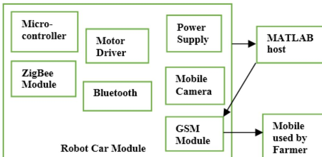
Fig. 9. Experiment setup diagram
