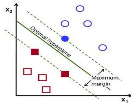
**Fig. 6.** Optimal separating hyperplane of SVM
