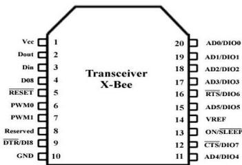
**Fig. 3:** Pin diagram of X-Bee Transceiver
