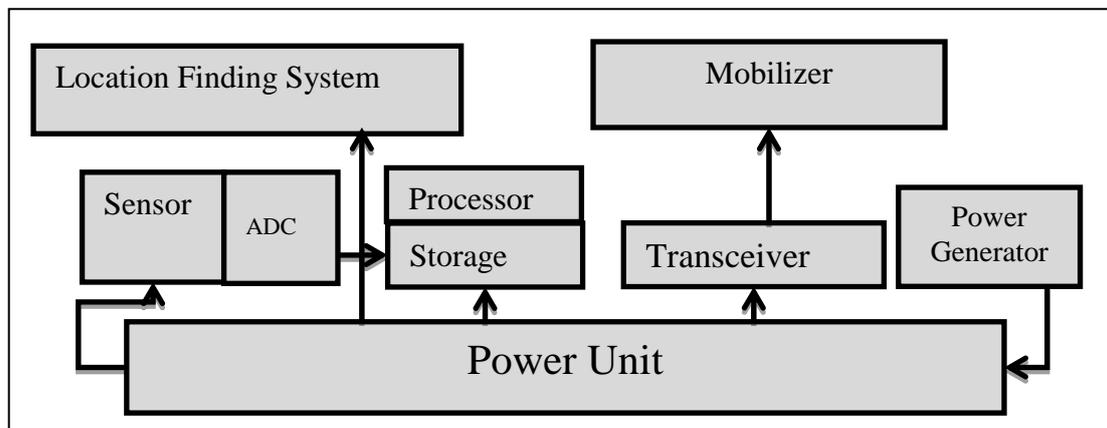
**Fig. 2** Components of a sensor node
