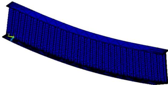
**Figure 9.** Deformation Of Plate Girder With 20mm Thick Corrugated Plate
