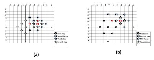
**Fig. 4.** An example of a search procedure for finding motion vector (3, -2) with (a) DS (b) HS. Each search point is indicated by its search step number and red colored point is the minimum search point.
