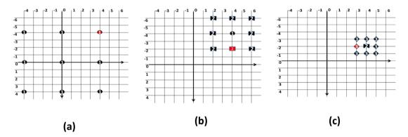
**Fig. 1.** The rectangular search patterns of TSS at (a) first search step (assume  $s = \pm 7$ ) (b) second search step, a rectangular search pattern is placed around minimum search point of first search step and step size is half of the first step (c) third search step, a rectangular search pattern is placed around minimum search point of second step and step size is half of the second step. The minimum search point is highlighted with red color.
