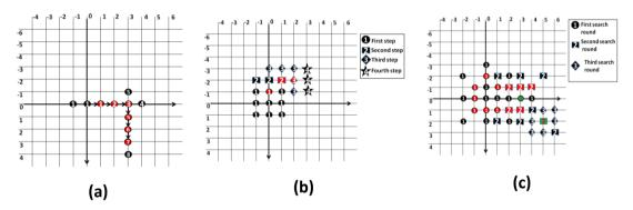
**Fig. 3.** An example of a search procedure of (a) OTS for finding motion vector (3, 3) (b) BBGDS for finding motion vector (2, -2) (c) DGDS for finding motion vector (5, 2). Each search point is indicated by its search step number and red colored point is the minimum search point.
