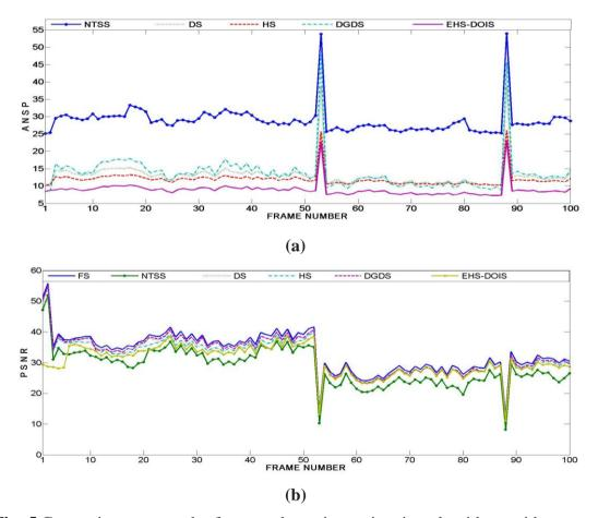
**Fig. 5.**Comparison among the fast search motion estimation algorithms with respect to (a) average number of search points (ANSP) per block and (b) average PSNR per frame with respect to full search algorithmfor "Flower" video sequence.
