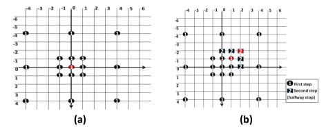
**Fig.2.** An example of a search procedure of NTSS for (a)a stationary block with (0,0) motion vector(b) a quasi-stationary block with motion vector (2, -2). Each search point is indicated by its search step number and red colored point is the minimum search point.
