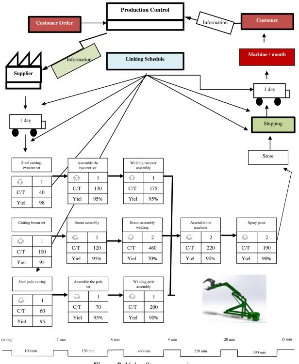
Figure 9. Value Stream mapping
