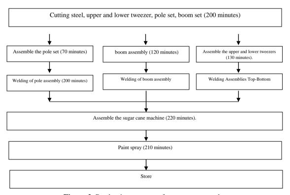
Figure 2. Production process of sugarcane grapple
