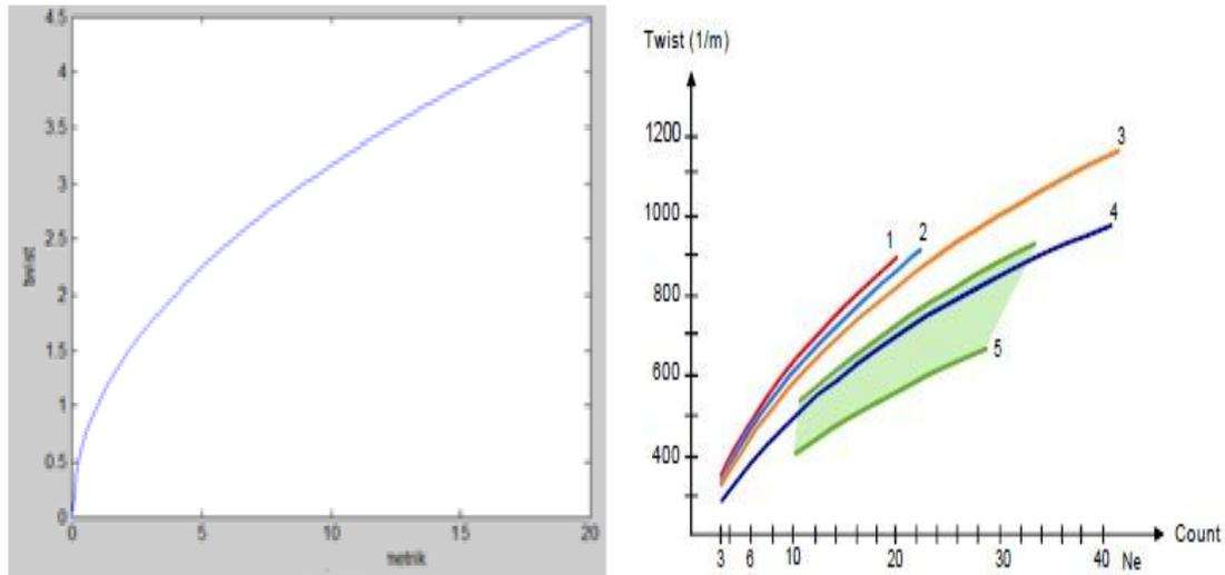
**Figure3:** Relationship of Twist and Yarn Count in Metric (Model and Furter’s Experiment)
