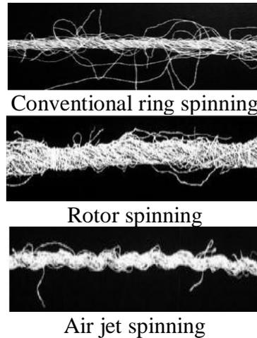
**Figure1:** Structure of Yarn Based on Machine Characteristic
