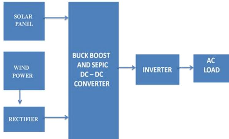
**Figure3.** Block diagram of proposed buck-Boost and SEPIC Converter
