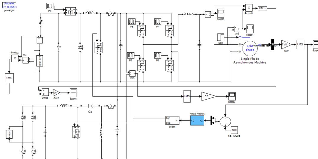
**Figure6.** Simulation for BUCK-BOOST and SEPIC converter
