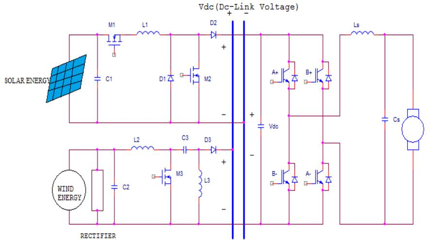
**Figure4.** Circuit diagram of proposed Buck-Boost and SEPIC converter
