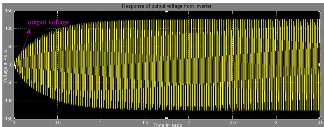
Figure9. Output voltage waveform of Inverter
