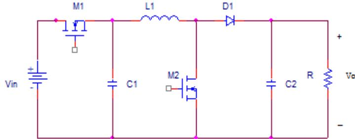
**Figure1.** Buck-Boost Converter
