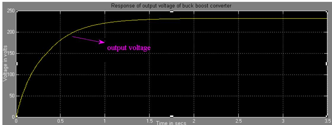
Figure7. Output voltage waveform of Buck-Boost converter operation
