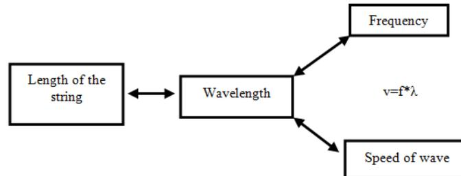
**Figure 6:** Relation between length, wavelength, frequency and speed of wave
