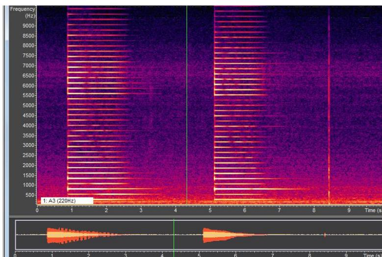
**Figure 27:** Two dimensional digital waveguide implementation of string with curved bridge and decay factor of 0.991 with pluck point at  $1/4^{\text{th}}$  length of the string and two dimensional digital waveguide implementation of string with curved bridge and decay factor of 0.991 with pluck point at center ( $1/2$  length of the string).
