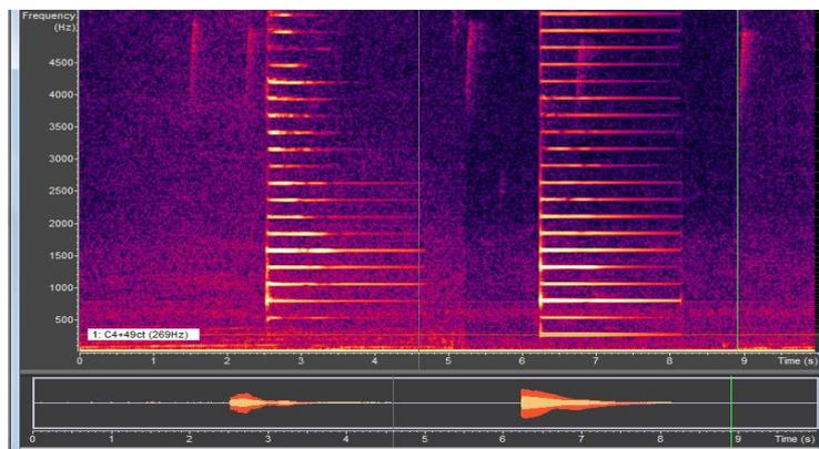
**Figure 22:** Actual Sitar tone plot along with one dimensional digital waveguide implementation of string with flat bridge and decay factor of 0.991 with pluck point at center ( $1/2$  length of the string)
