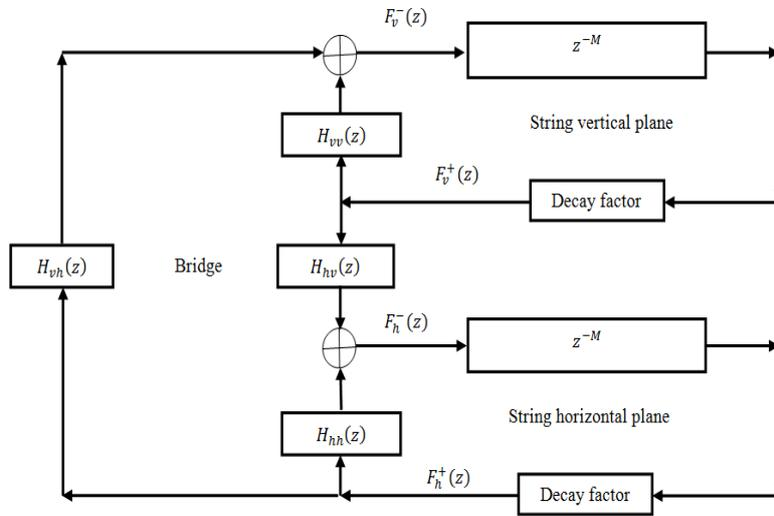
**Figure 15:** Coupling of the two vibration planes at the bridge
