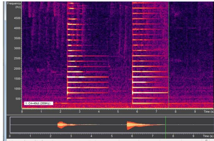
**Figure 18:** Actual Sitar tone plot along with FDM implementation of string with flat bridge structure and decay factor of 0.991 with pluck point at center (1/2 length of the string)
