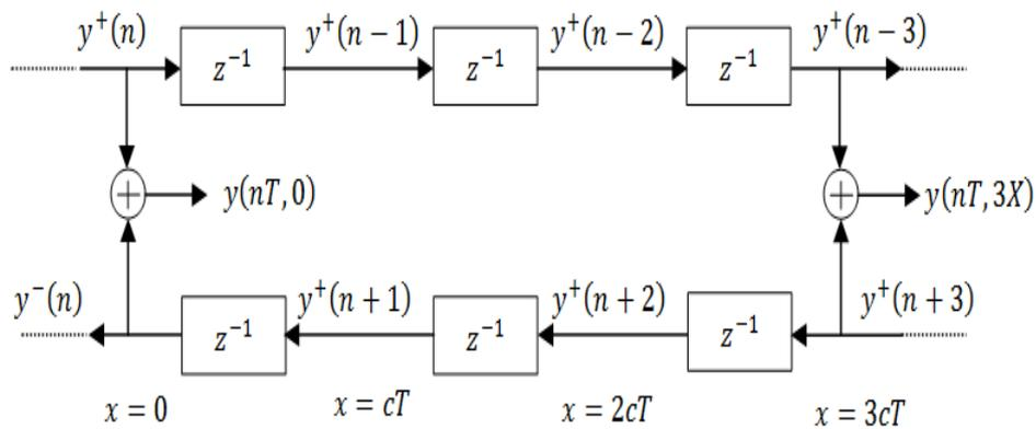
**Figure 10:** Digital representation of waveguide having ideal, lossless characteristics with three sample bidirectional delay line ( $z^{-1}$  represents one sample delay)
