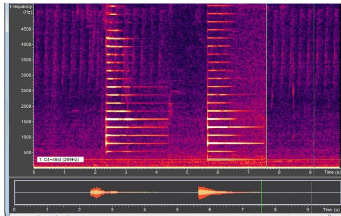
**Figure 19:** Actual Sitar tone plot along with FDM implementation of string with curved bridge structure and decay factor of 0.991 with pluck point at center (1/2 length of the string)
