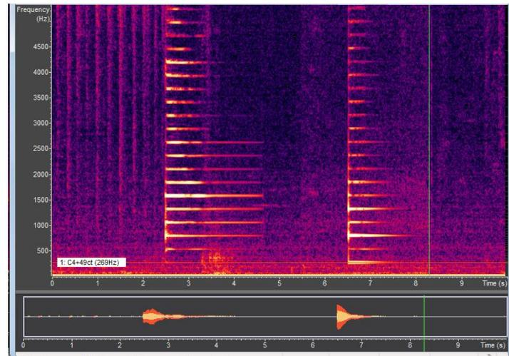
**Figure 17:** Actual Sitar tone plot along with FDM implementation of string with decay factor of 0.991 with pluck point at center (1/2 length of the string)
