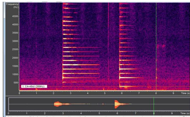
**Figure 21:** Actual Sitar tone plot along with one dimensional digital waveguide implementation of string with decay factor of 0.991 with pluck point at center ( $1/2$  length of the string)
