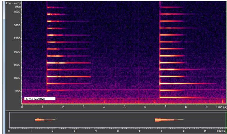
**Figure 25:** Actual Sitar tone plot along with two dimensional digital waveguide implementation of string with curved bridge and decay factor of 0.991 with pluck point at center (1/2 length of the string)
