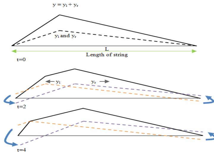
**Figure 12:** String shape determined by two traveling waves
