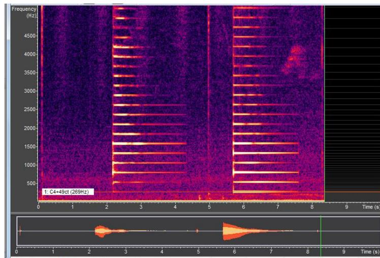
**Figure 24:** Actual Sitar tone plot along with one dimensional digital waveguide implementation of string with curved bridge and decay factor of 0.991 with pluck point at  $1/4^{\text{th}}$  length of the string
