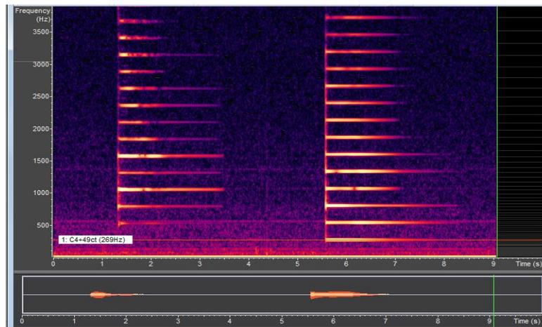
**Figure 26:** Actual Sitar tone plot along with two dimensional digital waveguide implementation of string with curved bridge and decay factor of 0.991 with pluck point at 1/4<sup>th</sup> length of the string
