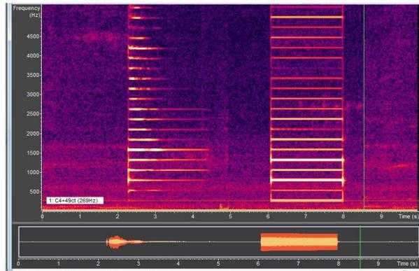
**Figure 20:** Actual Sitar tone plot along with one dimensional digital waveguide implementation of ideal string with pluck point at center ( $1/2$  length of the string)
