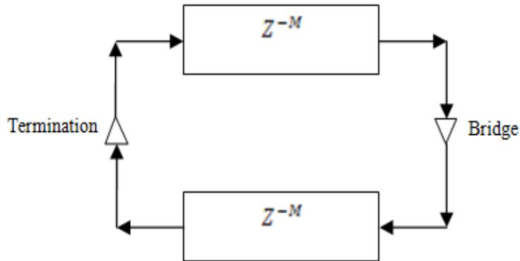
**Figure 11:** Digital representation of digital waveguide with  $2M$ -sample delay line
