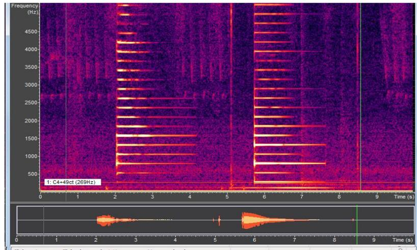
**Figure 23:** Actual Sitar tone plot along with one dimensional digital waveguide implementation of string with curved bridge and decay factor of 0.991 with pluck point at center ( $1/2$  length of the string)
