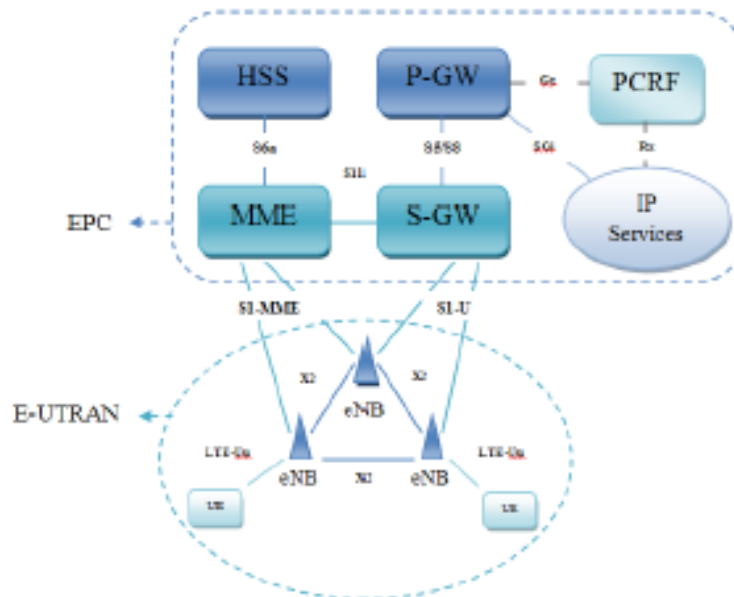
Figure 4: Evolved packet system
