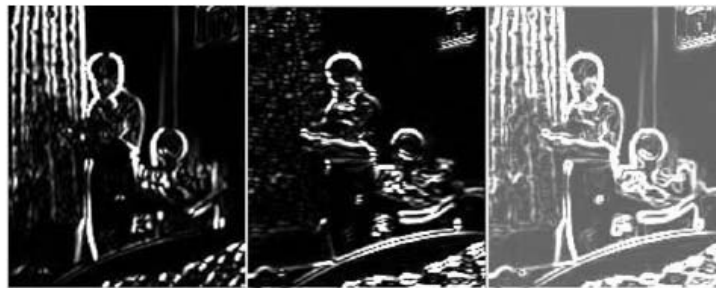
Figure 5: The first part shows the F_x^2 , second part is the F_y^2 and the last part is the summation of F_x & F_y with smoothness factor ^2 applied
