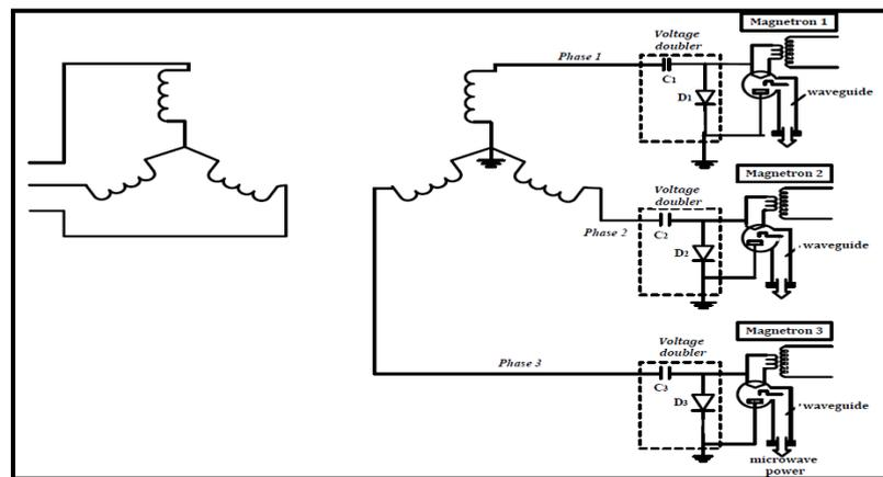
**Figure 1:** Three-Phase Power Supply For Magnetron By Phase
