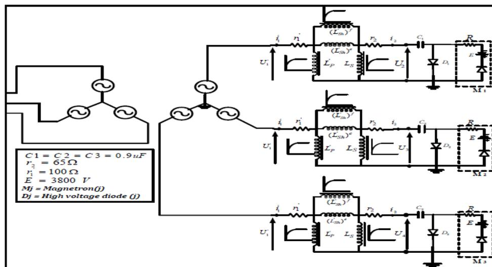
**Figure 3:** Three-Phase Power Supply Simulated By MATLAB SIMULINK Code
