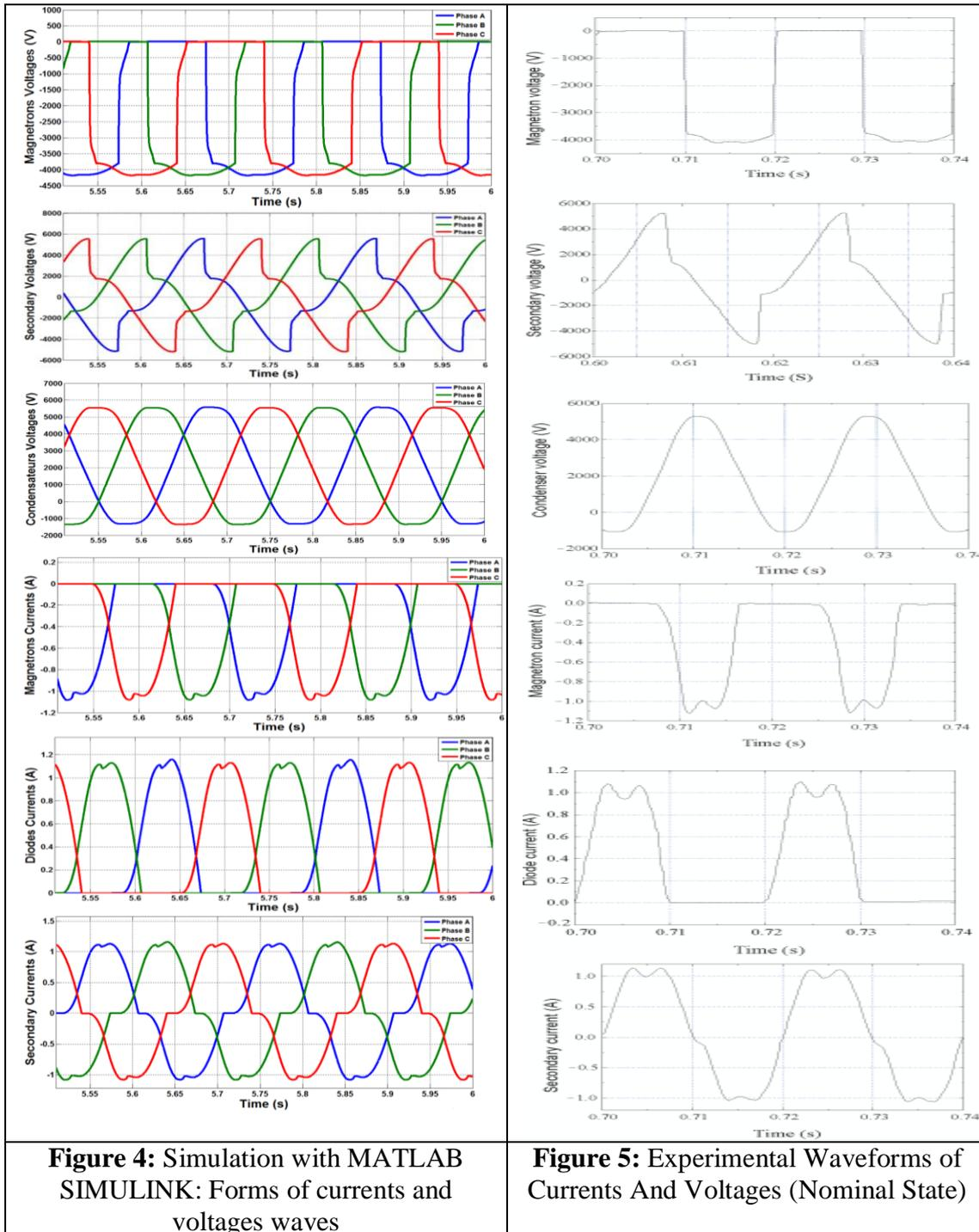
From the Fig.4 and Fig.5 we see that the signals obtained from simulation are curves of various sizes, periodic, non sinusoidal and dephasing by  $(2\pi/3)$  between them, which confirms the absence of interaction between magnetrons. These signals are in good accordance with those obtained by experimental and simulation of a conventional power supply using a single phase transformer for one magnetron [4].
