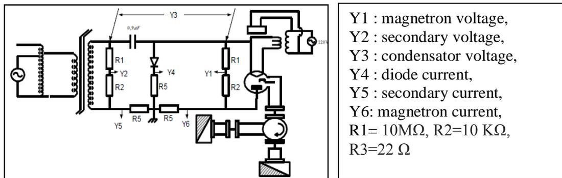
**Figure 6:** Experimental Set up for Measuring of the Characteristics:Current and Voltage of the Power Supply HV for Magnetron inNominal Operation
