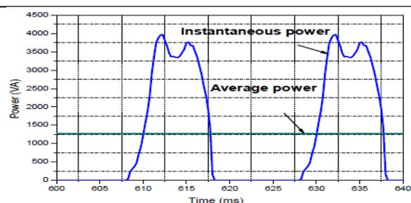
**Figure 8:** Average power and instantaneous power obtained by experimental of a single-phase power supply
