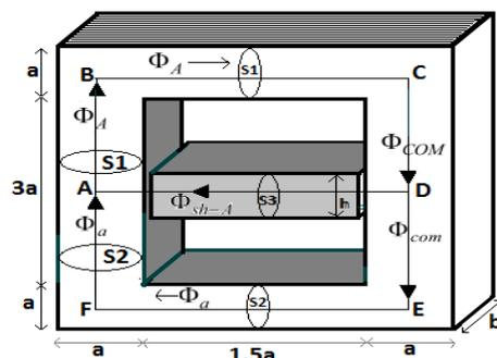
**Figure 9:** Geometry of Transformer With Magnetic Shunt (Phase A As Example)
