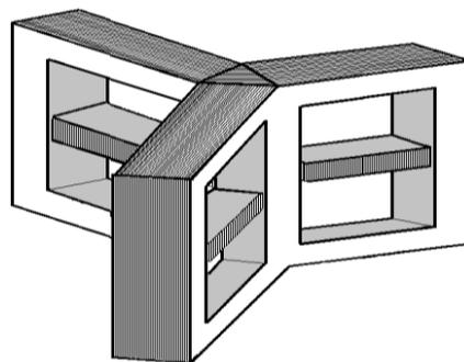
**Figure 2:** Equivalent Magnetic Circuit of The Three-Phase Transformer With Magnetic Shunt
