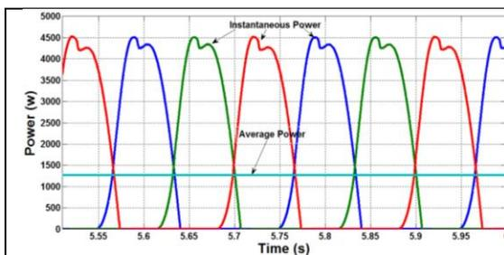
**Figure 7:** Average power and instantaneous power obtained by Matlab-Simulink for a three-phase power supply
