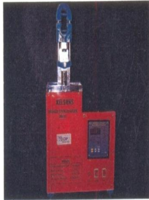
Figure 2: Universal sand strength Tensile test specimen machine along with tensile test attachment
