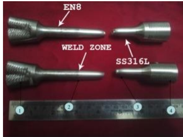
Fig.1. Fracture zone of the specimens after tensile testing
