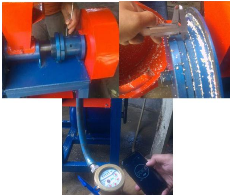
Figure 2: The component of regulation and measurement of the estrangement distance of the peeling wheel, flow meter and stopwatch on the test of machine performance
