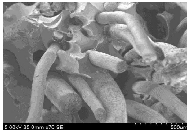
Figure 10: SEM micrograph illustrating vera fibre pull-out in Coir / Coir (Bi-directional) Composite
