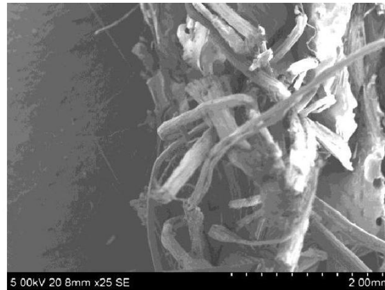
Figure 11: SEM micrograph of Aloe (random) composite showing interface debonding
