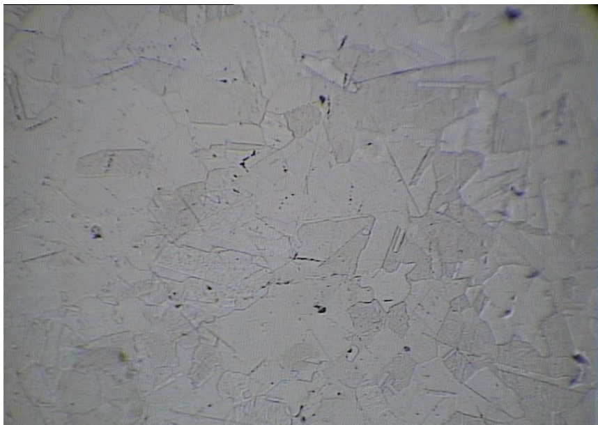
Figure 1 - Structure of pure lead Pb (20x42x8)
