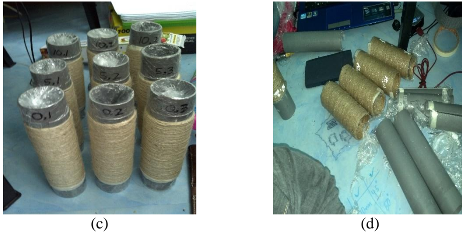
Fig. 3. (a) Plastic mould, (b) Mould assembly, (c) Kenaf yarn wrapped around the mould and (d) Final composite tubes.
