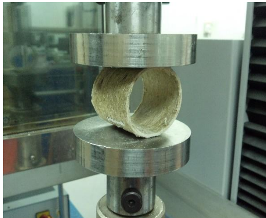
Fig. 4. Composite is laterally positioned before quasi-static compression loading.
