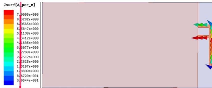
Figure 11: Current Distribution In Planar Inverted Folded Antenna At 2.4 GHz
