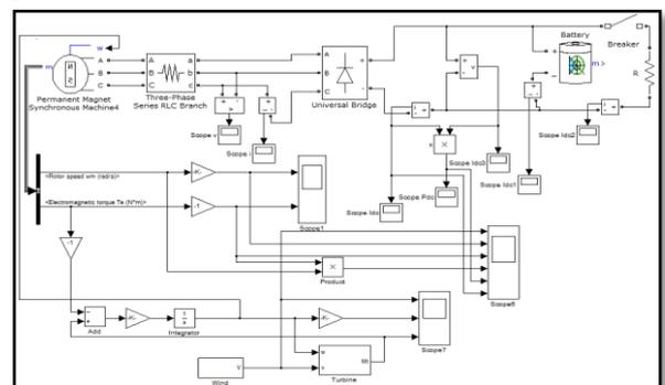
**Figure 1:** A computer simulation model of a hybrid WG. Computer simulation of wind wheel (windmill) operation in the form of torque to RPM rate at a given wind speed was made in the Simulink environment according to formulas (1) - (3) [8].
