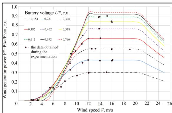
**Figure 2:** Power characteristics of WG with regard to the variation of nominal voltage of batteries obtained from simulation (lines) and experiments (stars)
