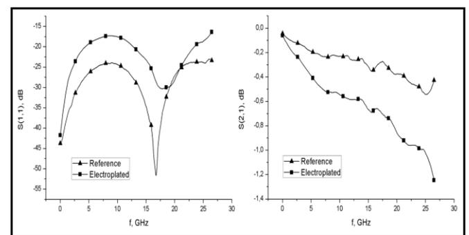
**Figure 1.1:** S-parameters of the reference (triangle) and the copper CPW on sapphire (square).
