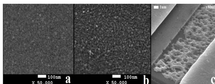
**Figure 1.4:** Effect of BHF on a copper film a) as deposited b) 10-minute BHF c) 10-minute BHF during SiO<sub>2</sub> etching.
