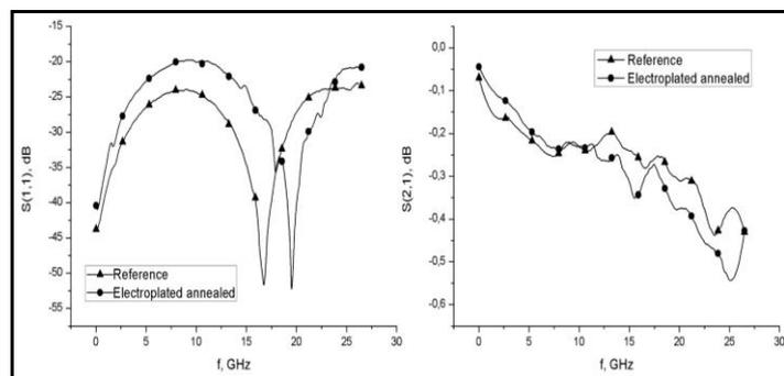
**Figure 1.2:** S-parameters of the reference (triangle) and the copper CPW on sapphire (square) after annealing.
