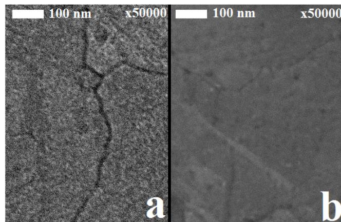
**Figure 1.5:** Effect of BHF and sputtered copper after annealing. a) sputtered copper, b) 10-minute BHF.
