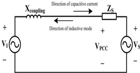
Figure 2: A DSTATCOM with a single phase power system.
