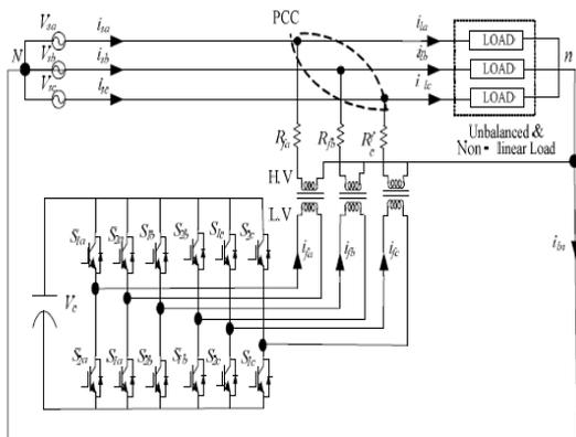
**Figure 8:** 3-independent single phase inverter with single dc capacitor based DSTATCOM
