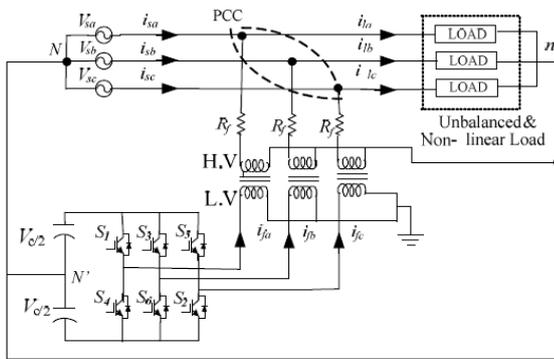
**Figure 7:** Split capacitor based DSTATCOM [28]
