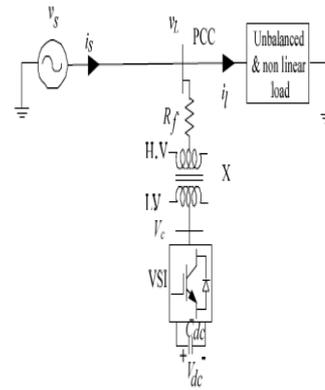
**Figure: 5** DSTATCOM structure for HV distribution system [28]
