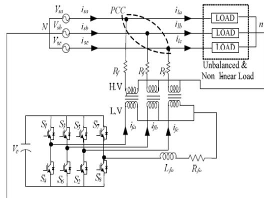
**Figure 9:** Three phase four leg inverter based DSTATCOM [28]
