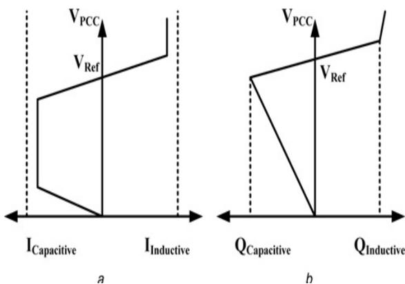
Figure 3: Shunt compensator operational characteristics (a) V-I (b) V-Q
