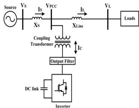
Figure 1: DSTATCOM Schematic diagram
