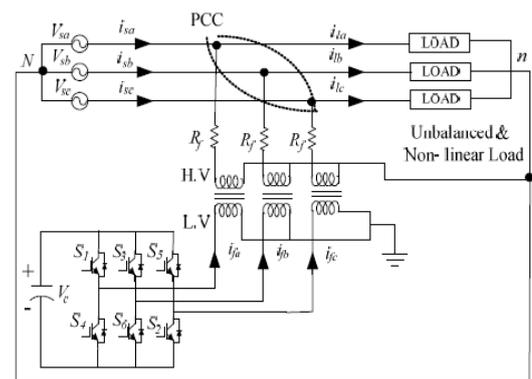
**Figure 6:** DSTATCOM (Three leg three phase inverter with a single dc capacitor) [28]
