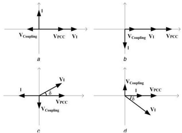
Figure 4: DSTATCOM different modes vector diagrams (a) Capacitive mode (b) Inductive mode (c) Active power release (d) Active power absorption.
