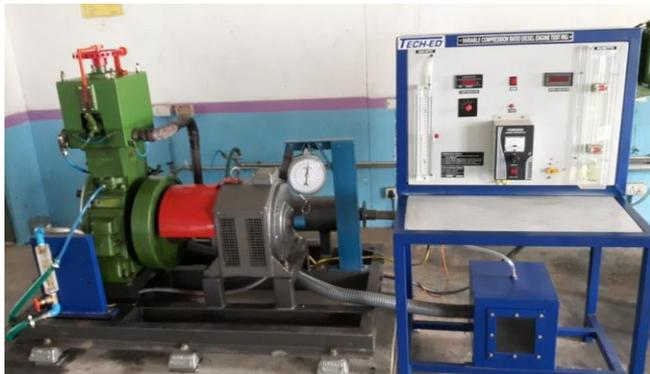
**Figure 1:** Experimental engine set up
