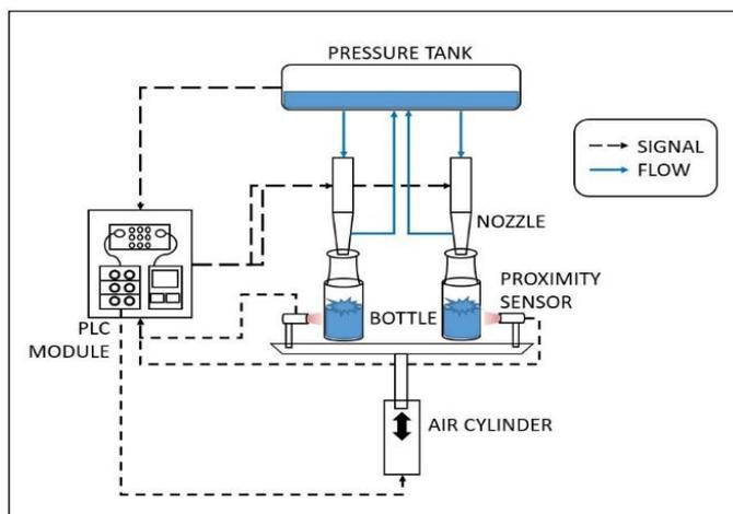
**Figure 2.** Schematic of the filling machine operating with PLC.
