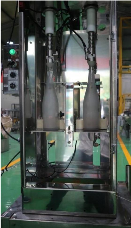
**Figure 1.** Prototype of industrial soda-filling machine.
