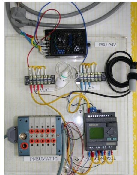
**Figure 3.** PLC module of the soda-filling machine.
