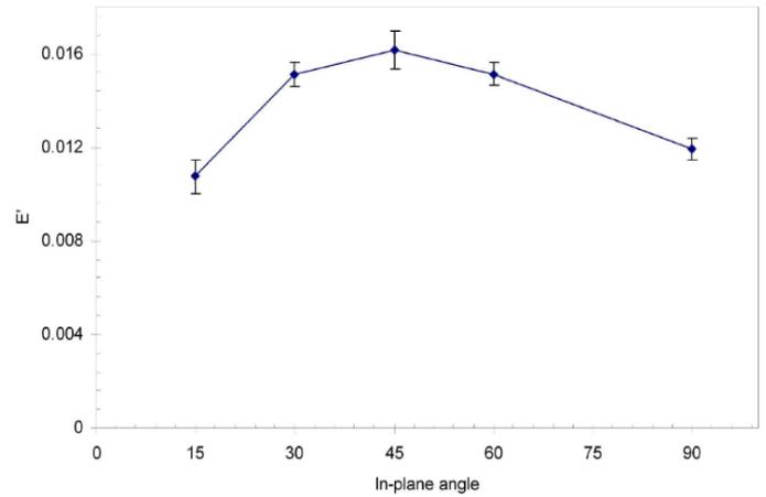
**Figure 7:** Effect of in-plane angle  $\theta$  on effective Young's modulus of 2D fiber networks of  $N = 900$ ,  $L = 0.25$ ,  $a = 25$ , and  $c_r = 0.5$ .
