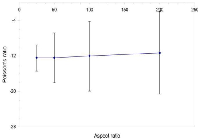
**Figure 8:** Effect of aspect ratio on Poisson's ratio of 2D fiber networks of  $N = 900$ ,  $L = 0.25$ ,  $\theta = \pm\pi/12$ , and  $c_r = 0.5$ .
