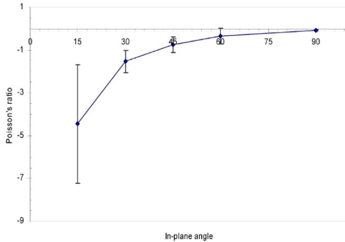
**Figure 6:** Effect of in-plane angle  $\theta$  on Poisson's ratio of 2D fiber networks of  $N = 900$ ,  $L = 0.25$ ,  $a = 25$ , and  $c_r = 0.5$ .
