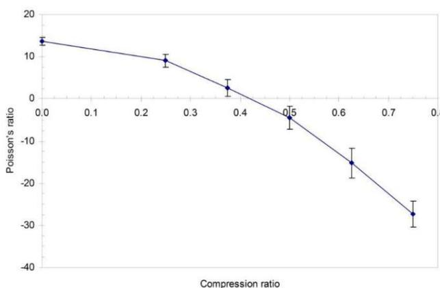
**Figure 4:** Effect of compression ratio on Poisson's ratio of 2D fiber networks of  $N = 900$ ,  $L = 0.25$ ,  $a = 25$ , and  $\theta = \pm\pi/12$
