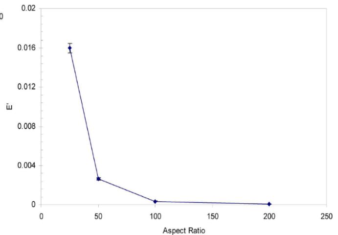
**Figure 9:** Effect of aspect ratio on effective Young's modulus of 2D fiber networks of  $N=900$ ,  $L=0.25$ ,  $\theta=\pm\pi/12$ , and  $c_r = 0.5$ .
