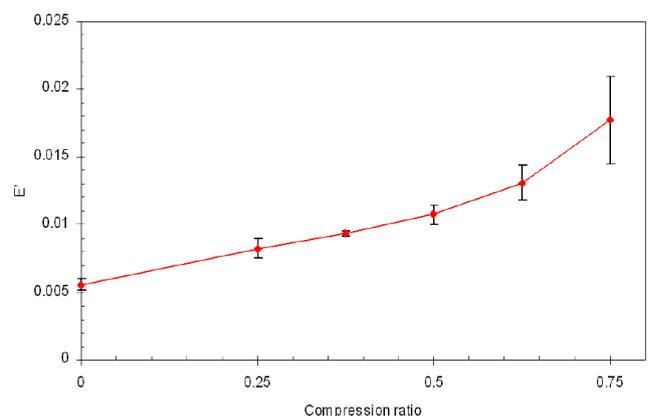
**Figure 5:** Effect of compression ratio on effective Young's modulus of 2D fiber networks of  $N = 900$ ,  $L = 0.25$ ,  $a = 25$ , and  $\theta = \pm\pi/12$ .
