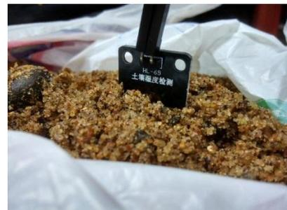
Figure 5: Moisture sensor in dry soil
