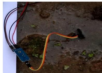
Figure 6: Moisture sensor in 100% moist condition
