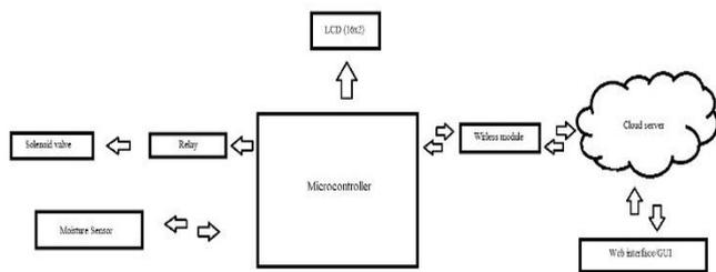
Figure 1: Block diagram of proposed hardware system components
