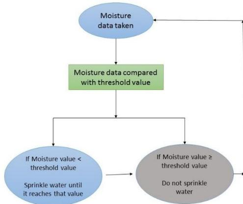
**Figure 8:** Basic algorithm for moisture control
