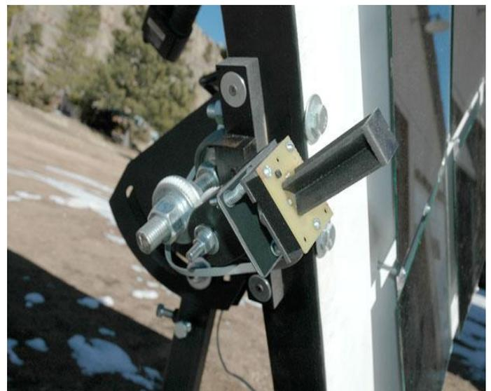
Sun Sensor used on Heliotrack's 1m by 1m heliostat.[9]
