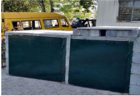
**Figure 10:** View of model buildings constructed for thermal study
