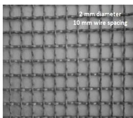
(a) Crimped steel mesh
