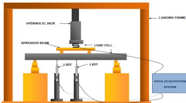
**Figure 3:** Schematic of flexure test setup
