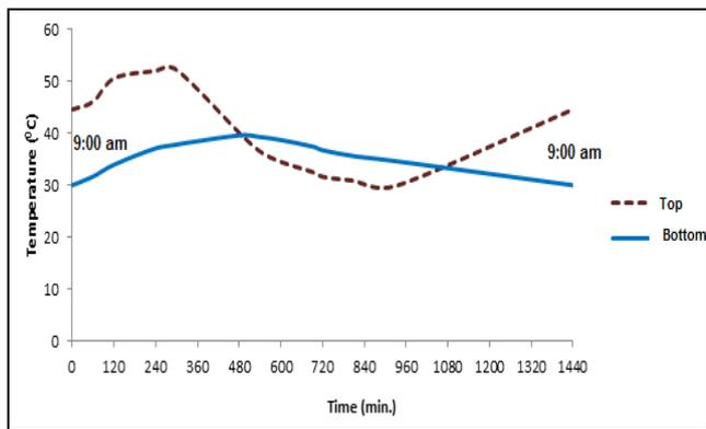
**Figure 23:** Hourly temperature variation in building with secondary roofing system for 24 hour period
