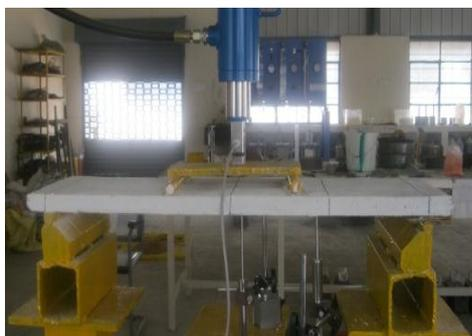
**Figure 4:** Flexure test in progress
