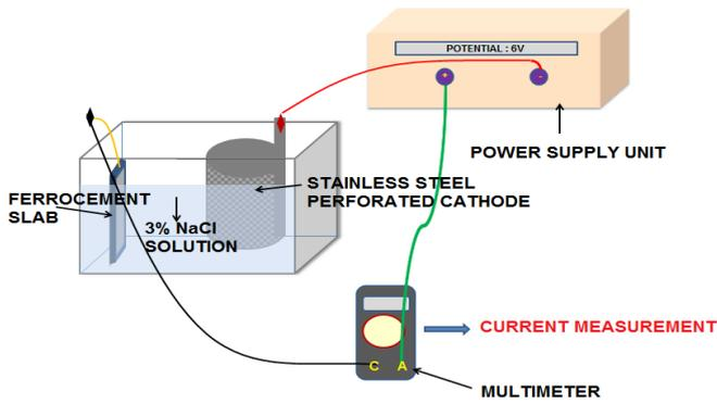
**Figure 6:** Schematic of the test set up for ACT
