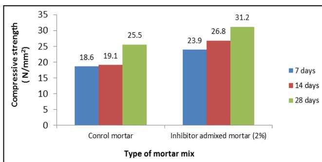
**Figure 11:** Comparison of compressive strength of control and inhibitor admixed mortar
