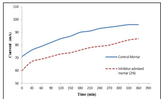
**Figure 16:** Time vs current behavior of control and inhibitor admixed mortar in RCPT
