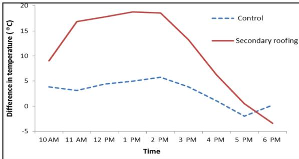
**Figure 19:** Time vs. average temperature difference values in model buildings
