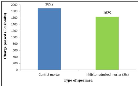
**Figure 17:** Comparison of charge passage for control and inhibitor admixed mortar in RCPT test
