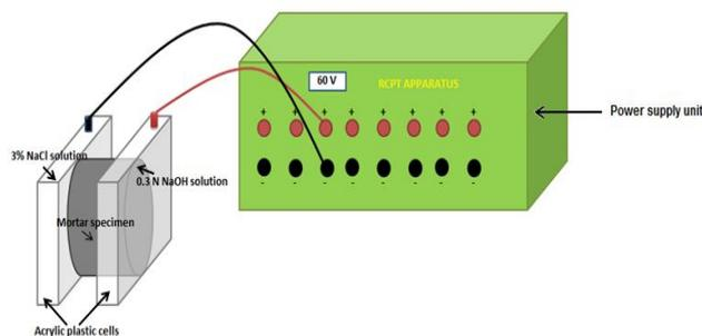
**Figure 7:** Schematic of rapid chloride penetration test (RCPT) setup
