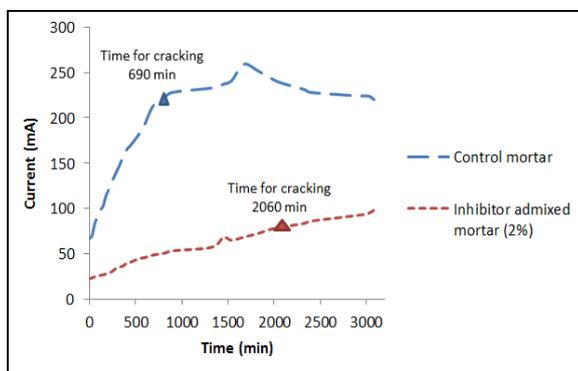
**Figure 15:** Time vs current behavior of control and inhibitor admixed ferrocement panels
