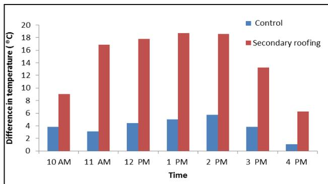
**Figure 20:** Comparison of difference in temperature in control and secondary roofing system
