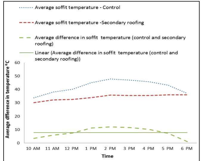
**Figure 21:** Average difference in temperature at soffit of slab in control and secondary roofing system
