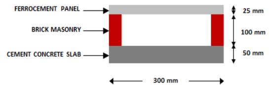
**(a) Ferrocement secondary roofing unit**
