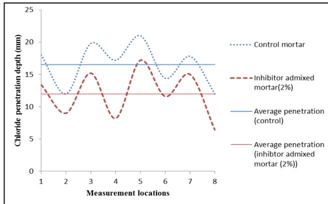
**Figure 14:** Chloride penetration behavior for control and inhibitor admixed mortar at various measurement locations
