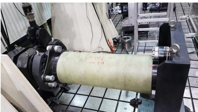
**Figure 13:** 6MW High Speed Coupling Fatigue Test
