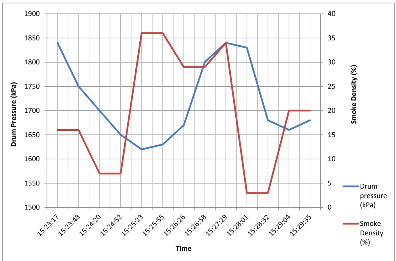
**Figure 1:** Drum pressure to the smoke density relationship
