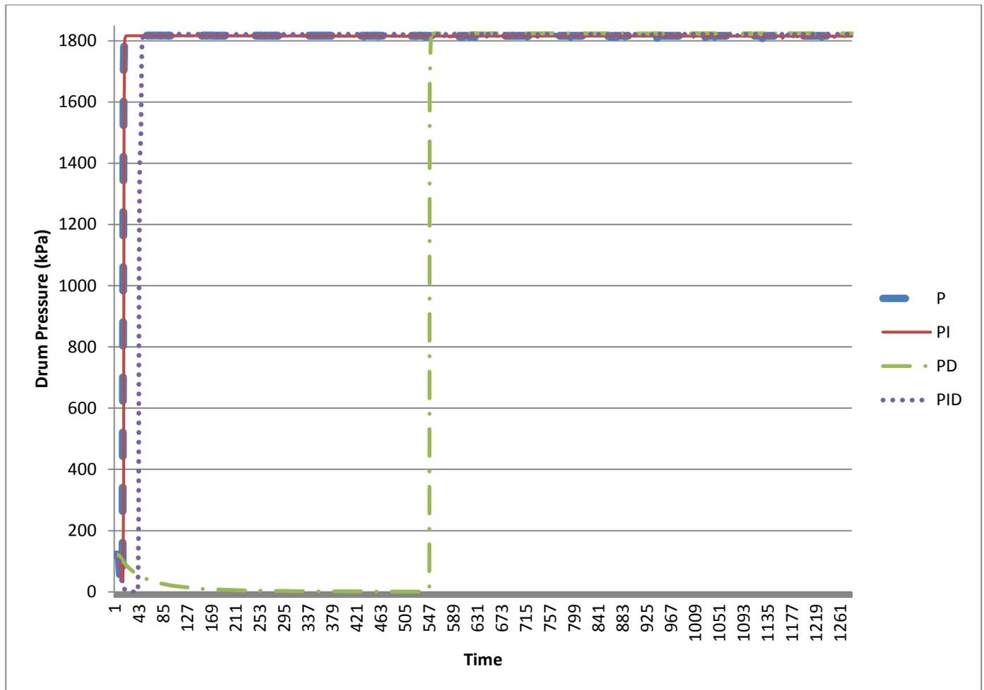
**Figure 3:** The boiler pressure responds of P controller, PI controller, PD controller and PID controller
