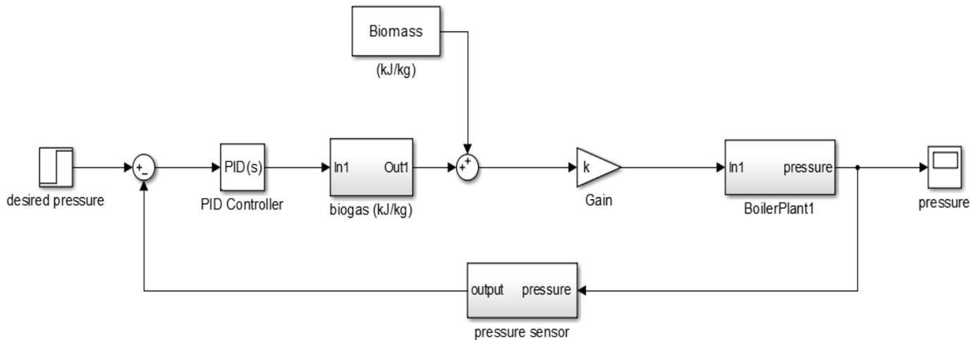
**Figure 2:** Block diagram of the feedback control
