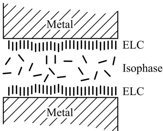
**Figure 2:** The structure of the narrow symmetric hetero-phase intermediate layer
