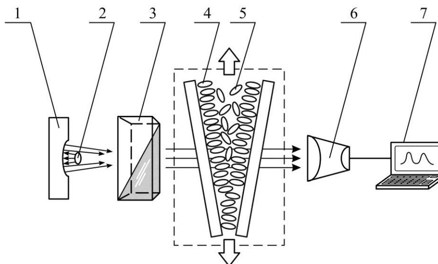
**Figure 4:** Scheme of scanning with the light probe of the wedge-shaped liquid layer:
