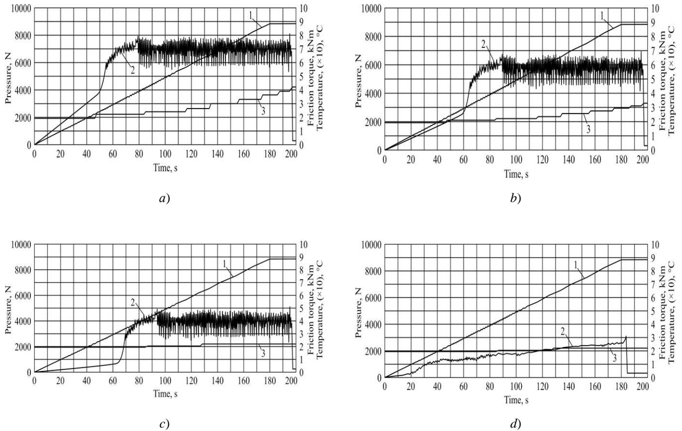
**Figure 5:** Friction machine test results for various LCLs
