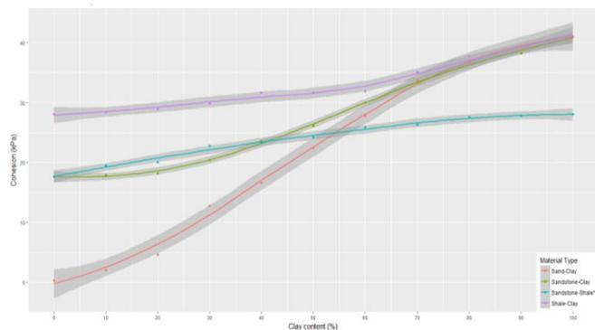
**Figure 2:** Cohesion vs clay (\*shale) content of mixed materials
