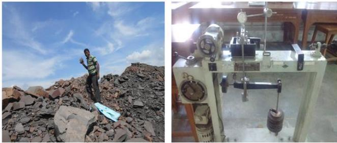
**Figure 1:** Sample collection and testing using small direct shear box
