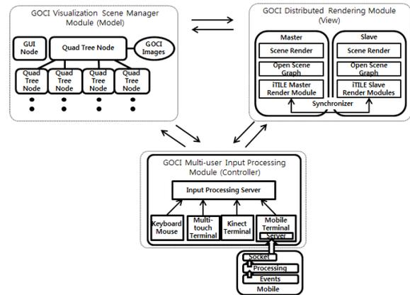
**Figure. 6** The Geostationary Ocean Color Imager (GOCI) visualization system consisting of the visualization scene manager, distributed rendering, and multi-user input processing modules
