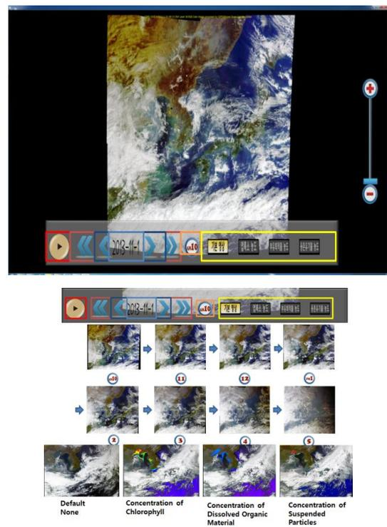
**Figure. 2** The main screen of the Geostationary Ocean Color Imager (GOCI) visualization with animation play/pause, date (month/day) change, and ocean state buttons (default none, concentration of chlorophyll, concentration of dissolved organic material, and concentration of suspended particles)
