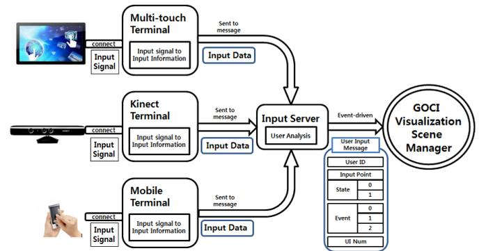
**Figure. 7** Input processing flow diagram for the multimodal user interaction
