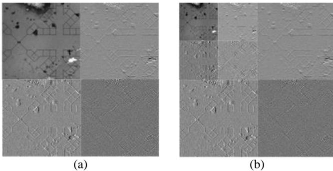
**Figure 3:** Decompositions of Fig. 2(b) using Haar wavelet at three decomposition levels: (a) first decomposition level; (b) second decomposition level.
