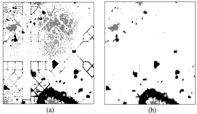
**Figure 5:** The resulting multiple level images of flaw detection with and without wavelet flat zone filtering: (a) without wavelet filtering; (b) with wavelet filtering.
