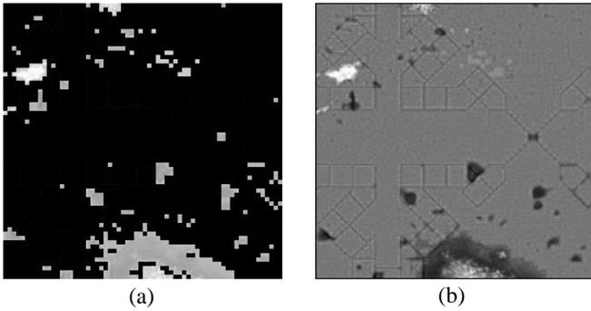
**Figure 4:** The reconstructed images with different flat zone filtering values: (a) frequency components replaced by zero; (b) frequency components replaced by mean value.
