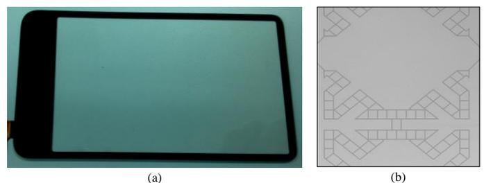
**Figure 1:** A TP screen with repeated pattern structure of sensing circuits and an enlargement of part of a TP surface.
