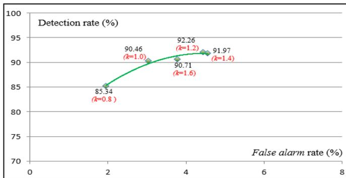
**Figure 7:** ROC plot of different zone sizes for wavelet filtering.
