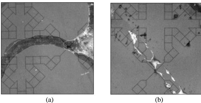
**Figure 2:** Two defective TP images with various area blemishes.
