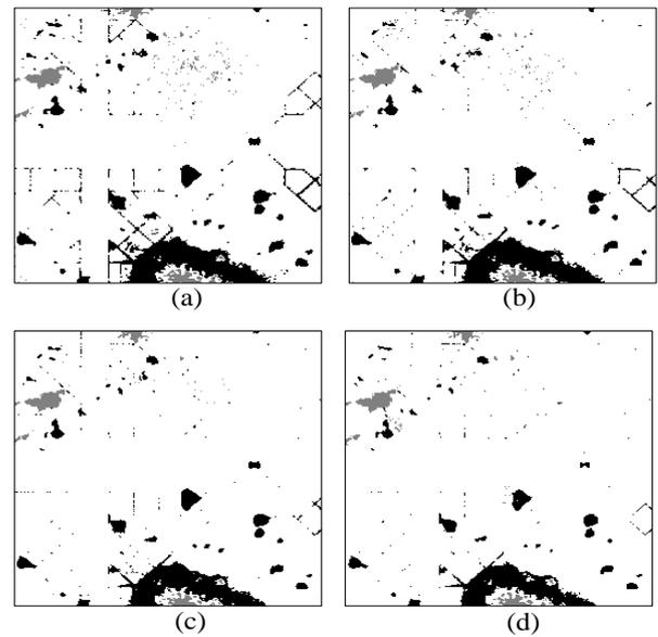
**Figure 6:** Resulting images of flaw detection at four wavelet decomposition levels: (a) first decomposition level; (b) second decomposition level; (c) third decomposition level; (d) fourth decomposition level.
