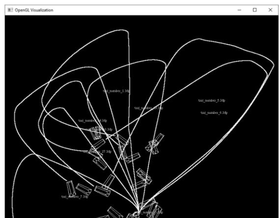
**Figure 9:** An example subset of successful trajectories for random ship dispositions during the neural network ship landing approach
