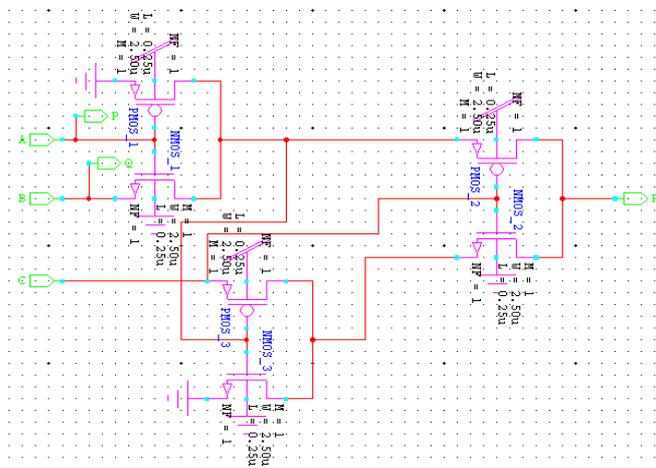
Figure 9: Schematic of Toffoli gate
