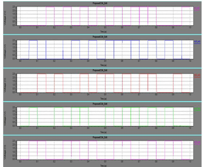
**Figure 31:** Output Simulation Results of Four bit Carry Skip Adder block using Peres, Toffoli and Fredkin gates
