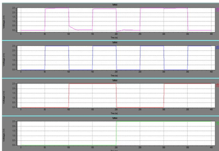
Figure 10: Simulation results of Toffoli gate
