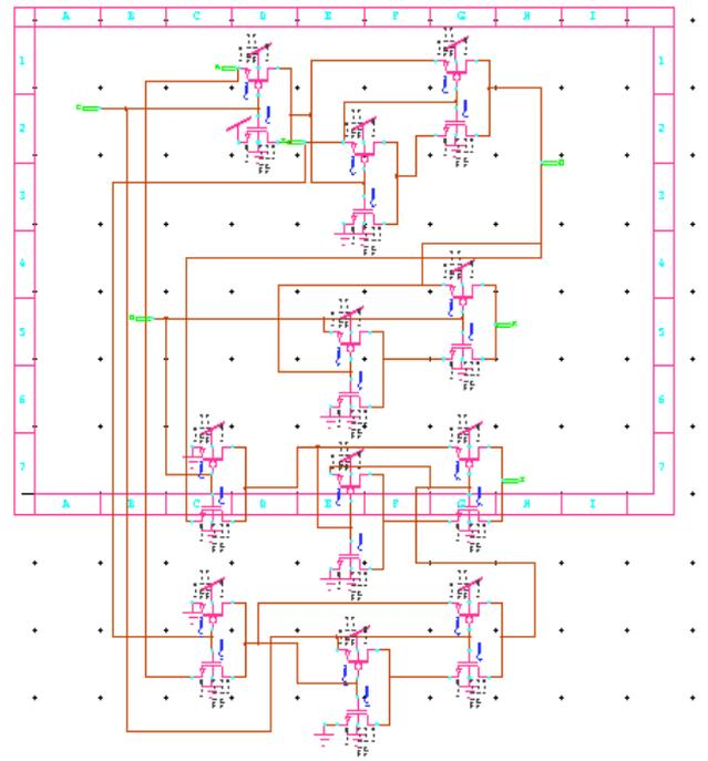
Figure 15: Schematic of TSG gate
