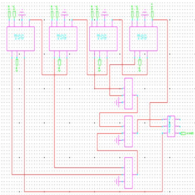
**Figure 18:** Transistor implementation of CSA using 4 TSG, 3 Toffoli and 1 Fredkin gates
