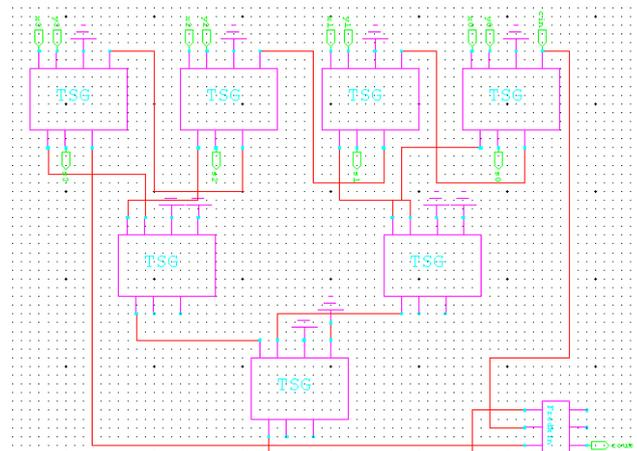
**Figure 22:** Transistor implementation of CSA using 7 TSG and 1 Fredkin gates
