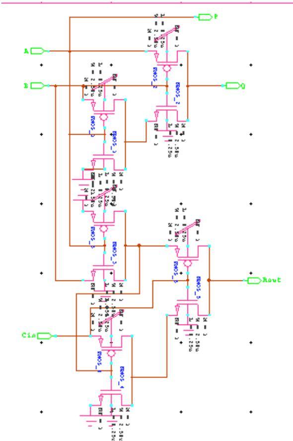
Figure 13: Schematic of Peres gate
