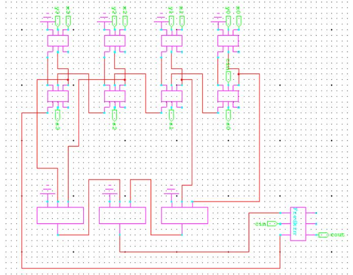
**Figure 30:** Four bit carry skip adder using Peres gates, Toffoli gates and Fredkin gate
