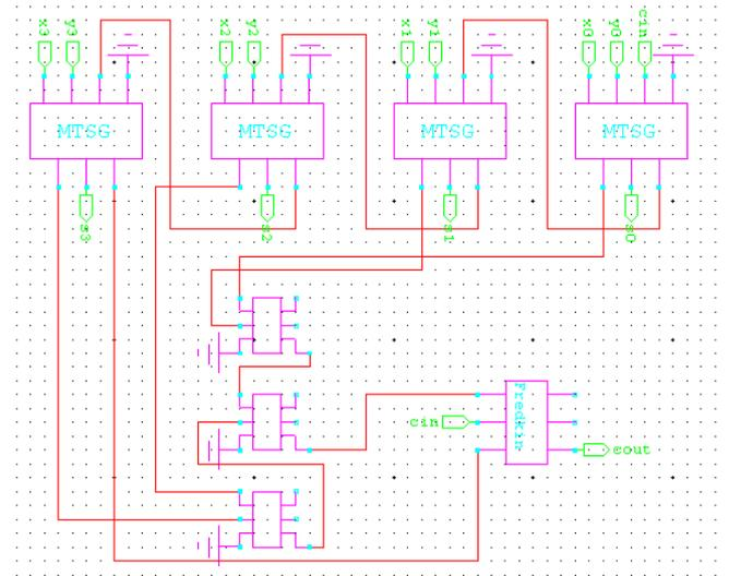
Figure 26: Transistor implementation of CSA using 4 MTSG, 3 Peres and 1 Fredkin gates
