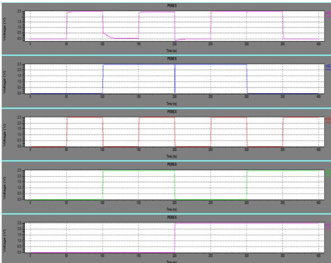
Figure 14: Simulation results of Peres gate
