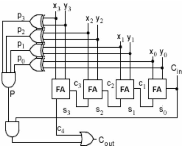
**Figure 29:** Four bit carry skip adder block [17]
