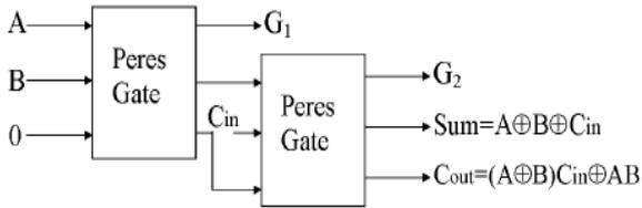
**Figure 28:** Block diagram of reversible full adder
