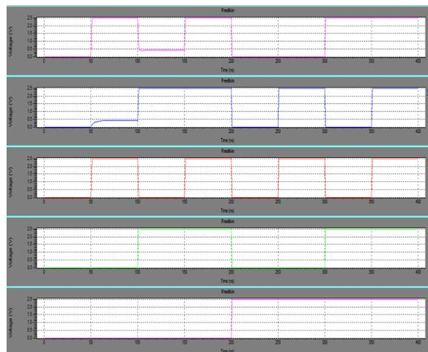
Figure 12: Simulation results of Fredkin gate
