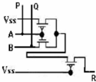
**Figure 17:** Transistor implementation of Toffoli gate as AND gate
