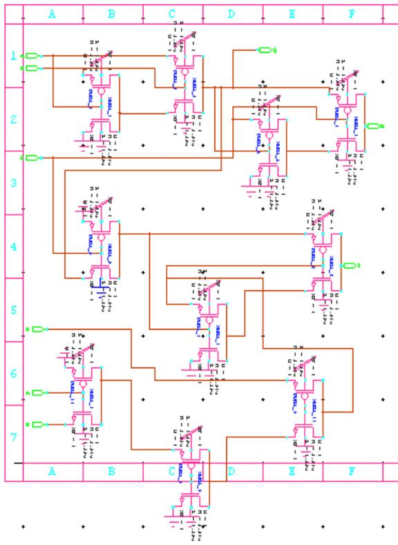
Figure 24: Transistor implementation of MTSG gate
