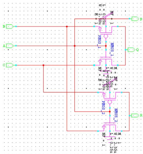
Figure 11: Schematic of Fredkin gate
