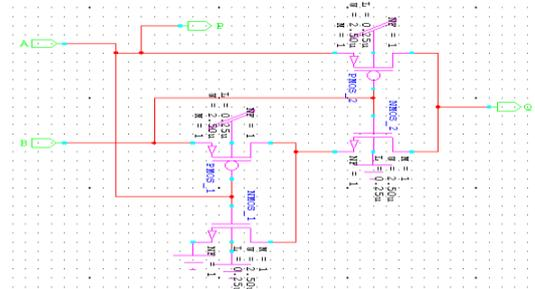
Figure 7: Schematic of Feynman gate
