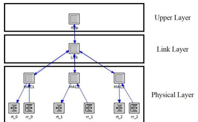
**Figure 3:** Simulation Architecture for BLE advertiser and scanner
