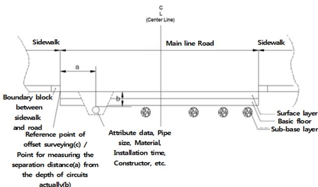
**Figure 3:** Offset surveying method
