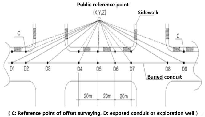
**Figure 4:** TS, GNSS surveying method
