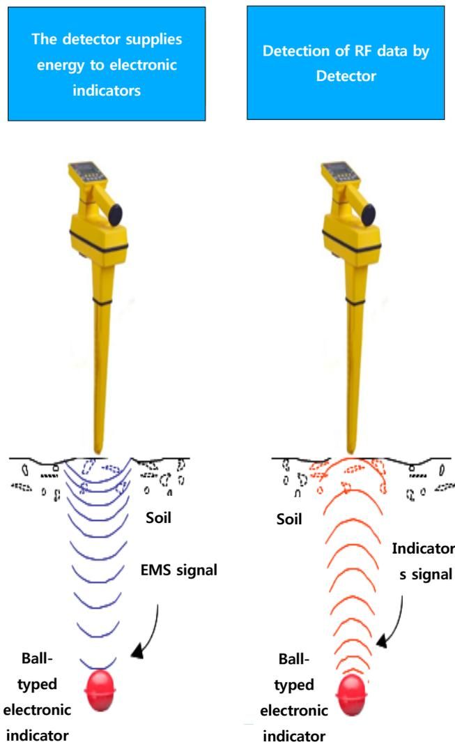
**Figure 2:** The principle of detecting conduits by using a detector and RF
