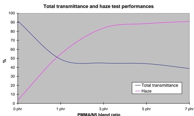
**Figure 10:** Characteristics of total transmittance and haze test
