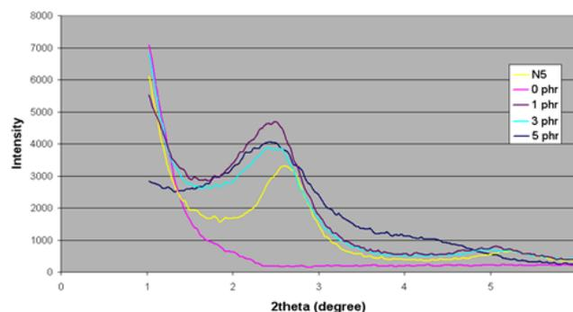
**Figure 2:** XRD Diffractogramme of various nanoclay content in PMMA matrix
