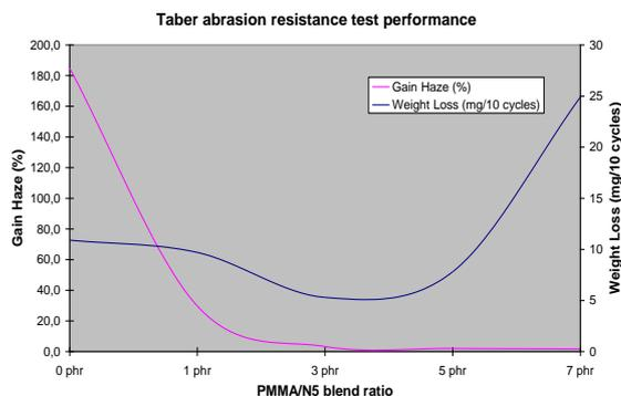
**Figure 13:** Evolution of the haze and the weight loss after Taber abrasion test.
