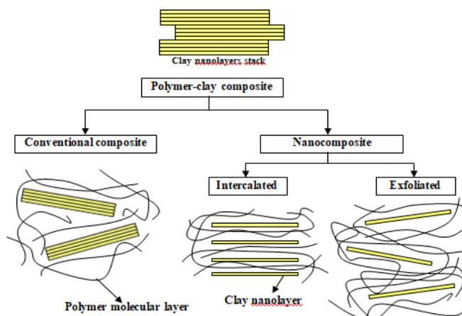
Figure 1: Structure of polymer-clay composite
