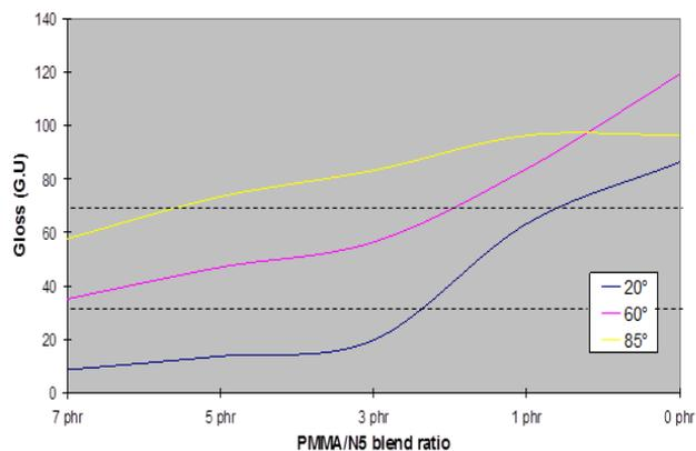
**Figure 11:** Characteristics of gloss test according to standard geometries 20°, 60° and 85°
