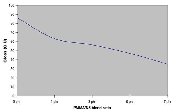
**Figure 12:** Characteristics of gloss test according to standard ASTM
