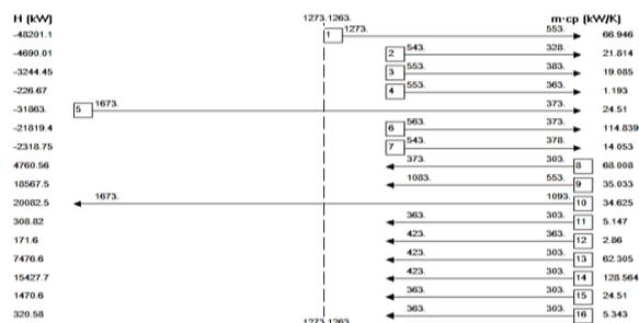
Figure 5: Grid Representation of the Process Stream
