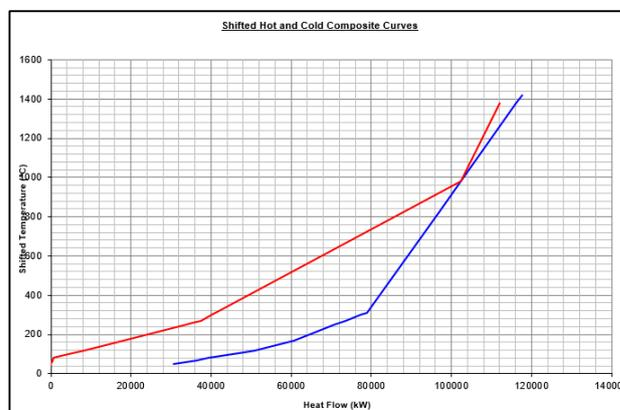
**Figure 3:** Hot and Cold Composite Curves without shifting considering  $\Delta T_{min} 0^\circ C$
