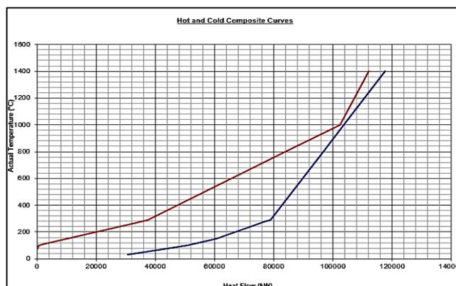
**Figure 2:** Hot and Cold Composite Curves without shifting considering  $\Delta T_{min} 10^\circ C$
