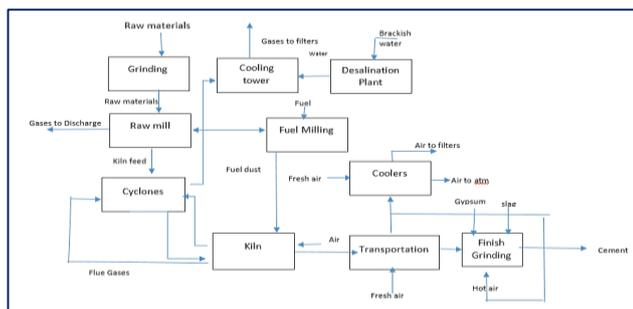
**Figure 1:** Cement Production Process
