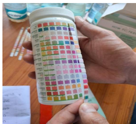
Figure.4: Strip compare with color chart
