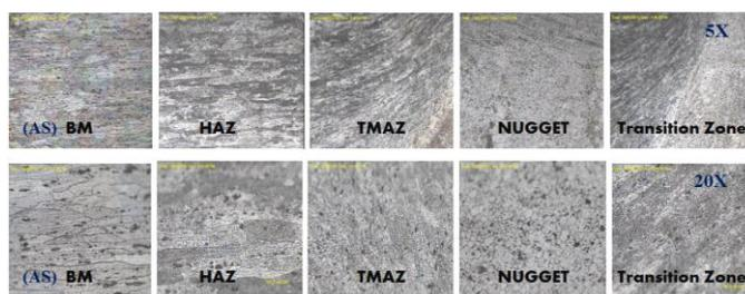
**Figure 8:** Enlarged micrographs for the locations indicated with 5X magnification in the upper row and 20X magnification in bottom row for rotation and traverse speed of 1400 rpm, 0.8 mm/s in the advancing and retreating sides. (high rotation speed with low traverse speed)
