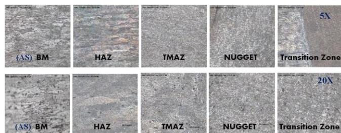
**Figure 5:**Micrographs for the locations indicated with 5X magnification (upper row) and 20X magnification (bottom row) for rotation and traverse speed of 650 rpm, 0.8 mm/s in the advancing side (AS). (low rotation speed and low traverse speed)
