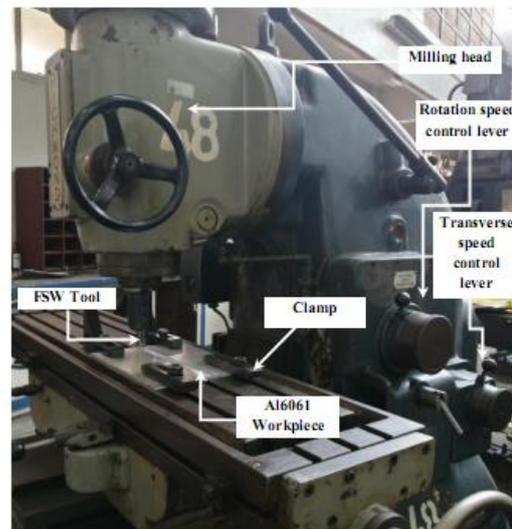
**Figure 2:** Friction stir welding process using a conventional milling machine
