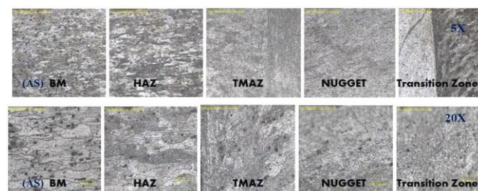
**Figure 6:** Micrographs for the locations indicated with 5X magnification ( upper row) and 20X magnification (bottom row) for rotation and traverse speed of 650 rpm, 4.55 mm/s in the advancing and retreating sides. (low rotation speed and high traverse speed)
