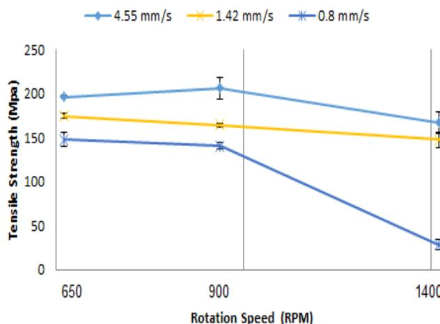
**Figure 10:** Tensile strength of varied FSW parameters with constant traverse speed and increased rotation speed with Error bars indicating a 95% confidence limit
