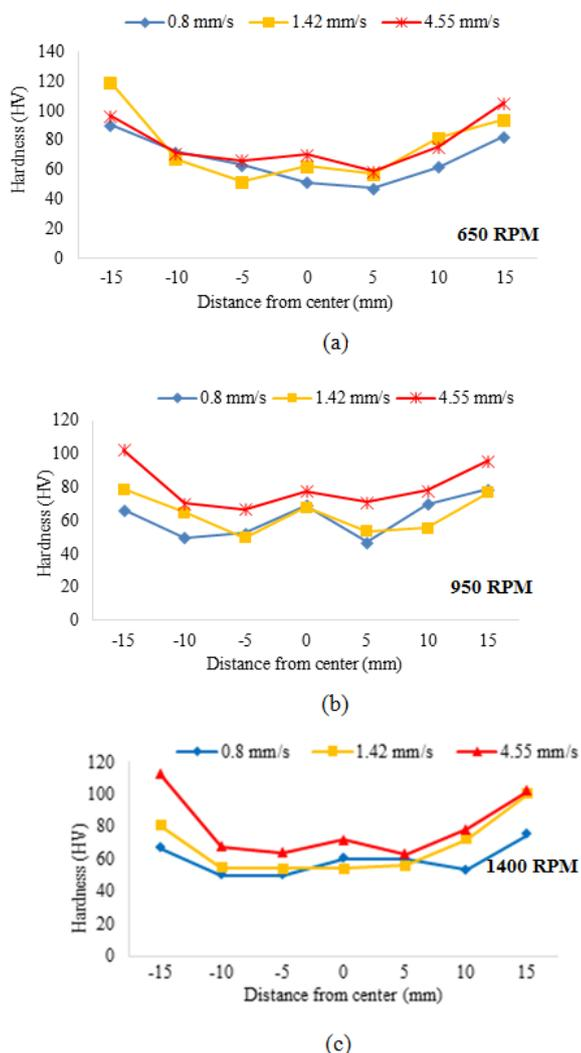
**Figure 11:** Friction Vickers hardness profiles in the weld zone and parent material for different variations of rotations speed (a) 650 rpm (b) 950 rpm and (c) 1400 rpm
