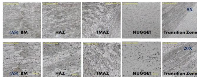
**Figure 7:** Micrographs for the locations indicated with 5X magnification ( upper row) and 20X magnification (bottom row) for rotation and traverse speed of 950 rpm, 4.55 mm/s in the advancing and retreating sides. (moderate rotation speed with high traverse speed)
