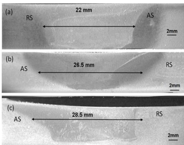
**Figure 3:** Transverse section macrographs for the joints obtained at the welding speed of 0.8 mm/s: (a) 650 rpm, (b) 950 rpm, and (c) 1400 rpm
