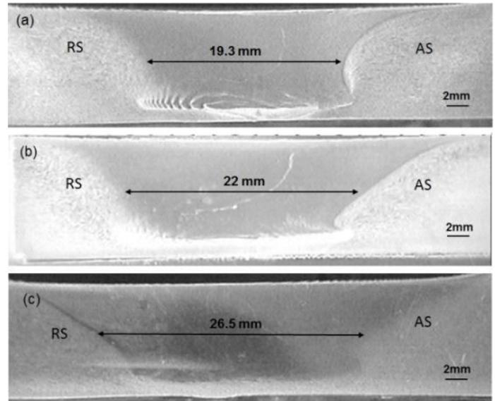
**Figure 4:** Traverse section macrographs for the joints obtained at the welding speed of 1.42 mm/s: (a) 650 rpm, (b) 950 rpm, and (c) 1400 rpm
