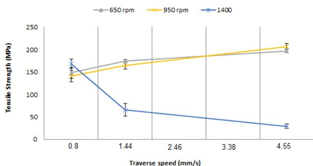
**Figure 9:** Tensile strength of varied FSW parameters with constant rotation speed and increased traverse speed with Error bars indicating a 95% confidence limit
