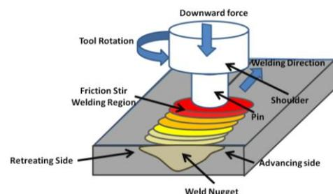
**Figure 1:** The friction stir welding process
