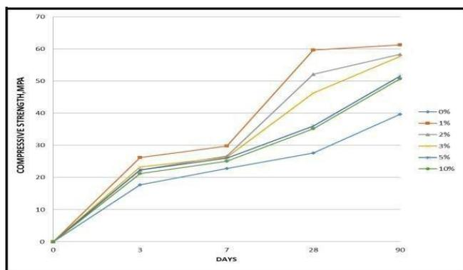
**Figure 2:** Compressive strength of control mix and polymer diapers concrete
