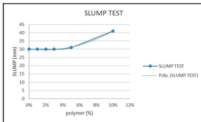
**Figure 1: Workability of concrete**
