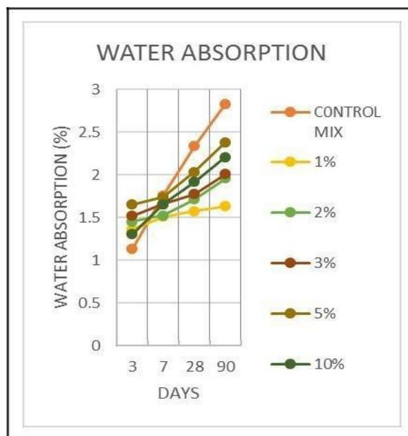
**Figure 3:** Water absorption against percentage of polymer replacement
