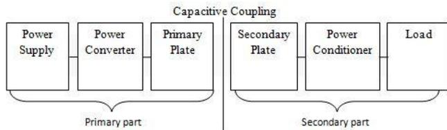
Figure 1. Block Diagram for Capacitive Power Transfer
