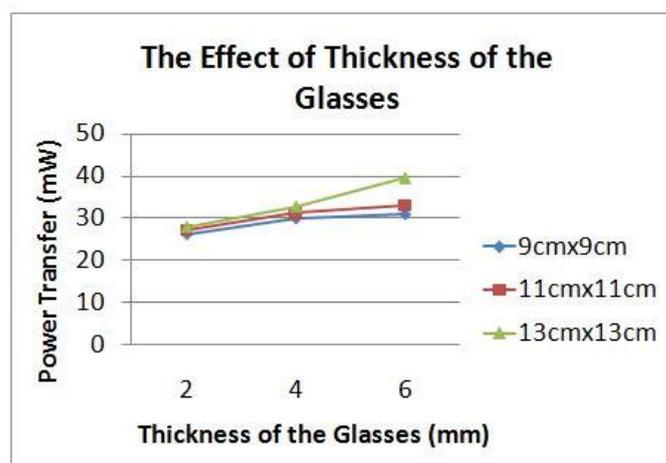
**Figure 19.** Power Transfer for the Different Thickness of the Glasses
