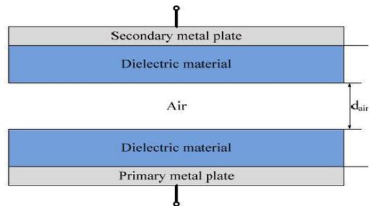
Figure 5. Schematic diagram of coupling with dielectric and air gap
