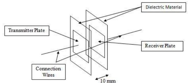
Figure 2. Schematic diagram of the distance between transmitter and receiver.
