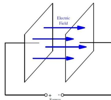
Figure 6. Schematic diagram of electric field coupling between two parallel plates
