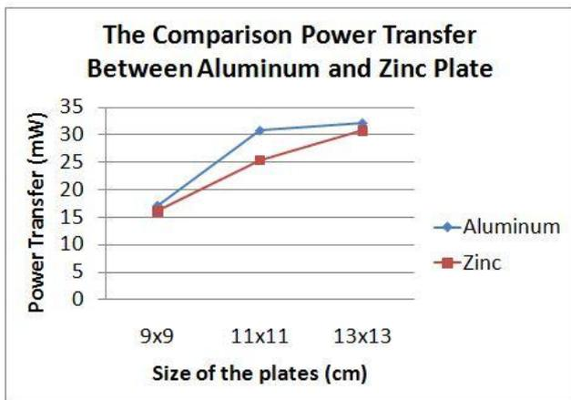
**Figure 20.** Graph between power transfer and for the size of the coupling plates
