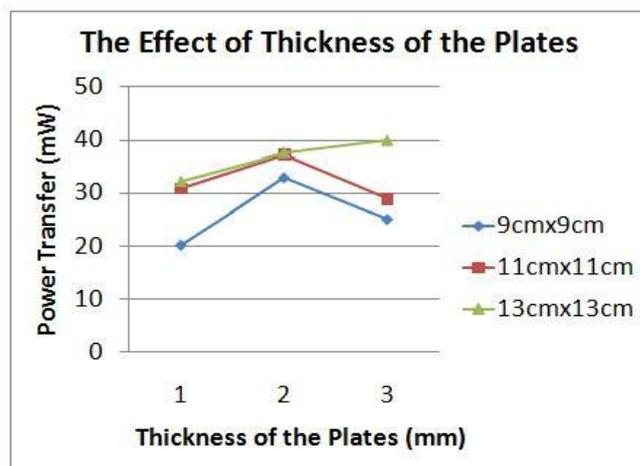
**Figure 18.** The graph between power transfer and thickness of the plate
