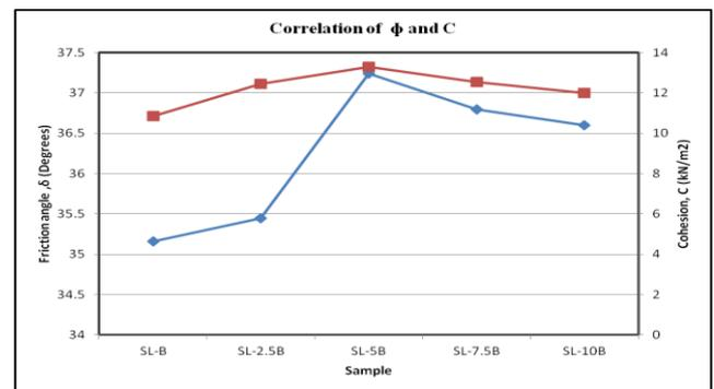
Figure 13: Correlation of friction angle and cohesion
