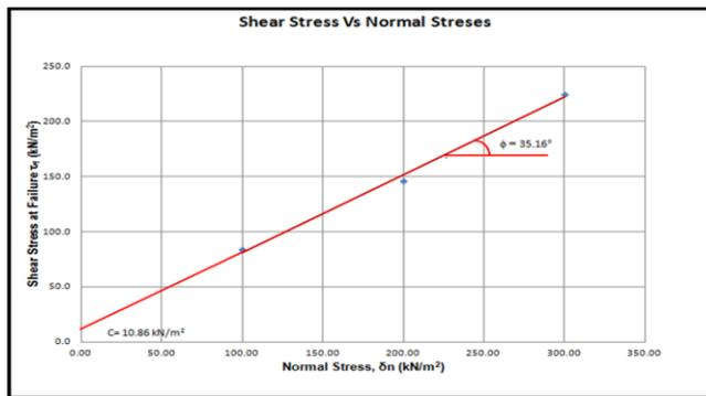
Figure 4: Graph of maximum shear stress vs normal stress for SL-B
