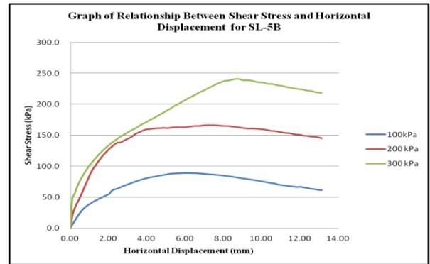
Figure 7: Graph of interface shear strength for SL-5B
