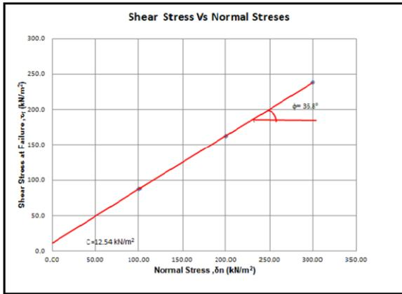
Figure 10: Graph of maximum shear stress vs normal stress for SL-7.5B
