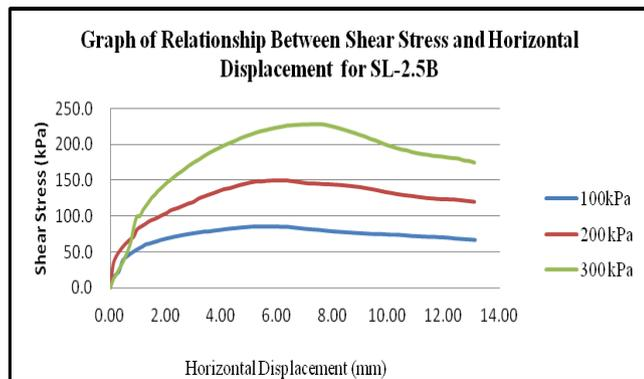
Figure 5: Graph of interface shear strength for SL-2.5B
