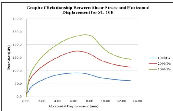
Figure 11: Graph of interface shear strength for SL-10B
