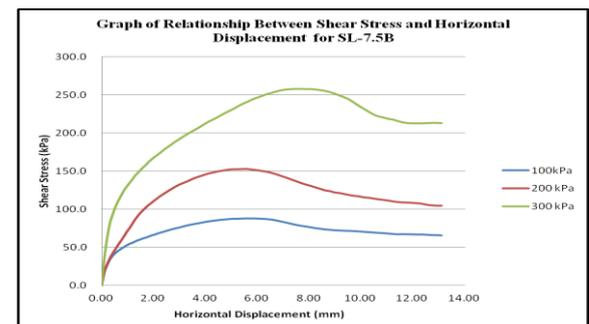
Figure 9: Graph of interface shear strength for SL-7.5B
