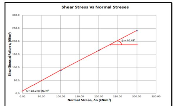
Figure 8: Graph of maximum shear stress vs normal stress for SL-5B
