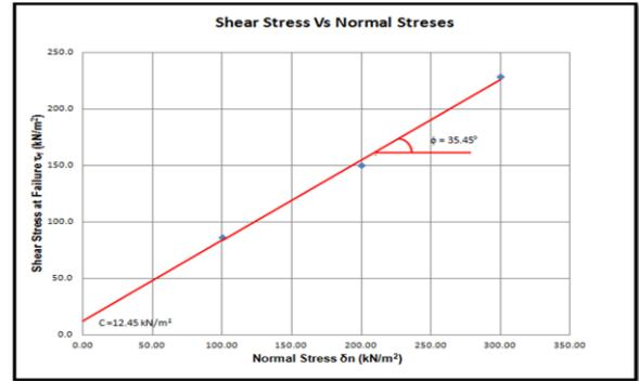
Figure 6: Graph of maximum shear stress vs normal stress for SL-2.5B
