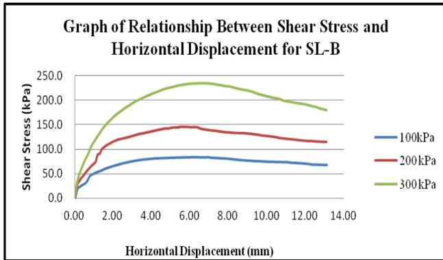
Figure 3: Graph of interface shear strength for SL-B
