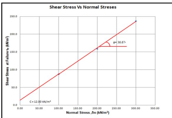
Figure 12: Graph of maximum shear stress vs normal stress for SL-10B
