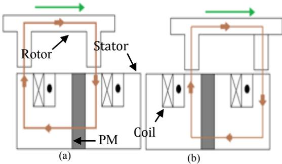
**Figure 1:** Operating principle of PMFSM
