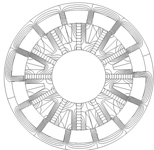
**Figure 5:** Outer rotor PMFSM flux lines
