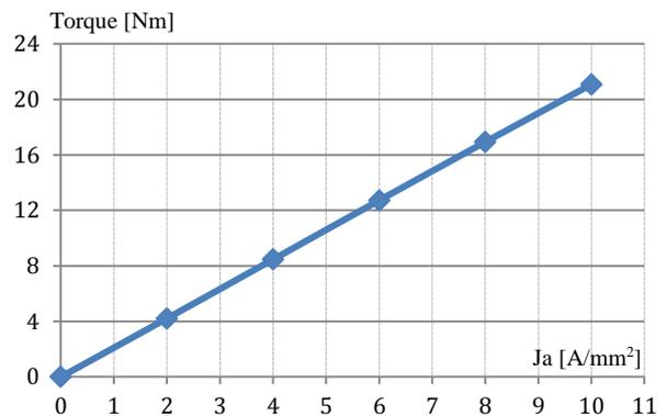
**Figure 9:** Torque versus various armature current densities
