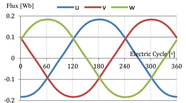
**Figure 4:** Three phase flux linkage
