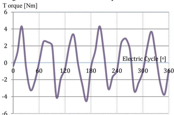
**Figure 7:** Cogging torque waveform
