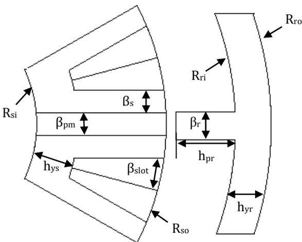
**Figure 2:** Key design parameters of outer rotor PMFSM
