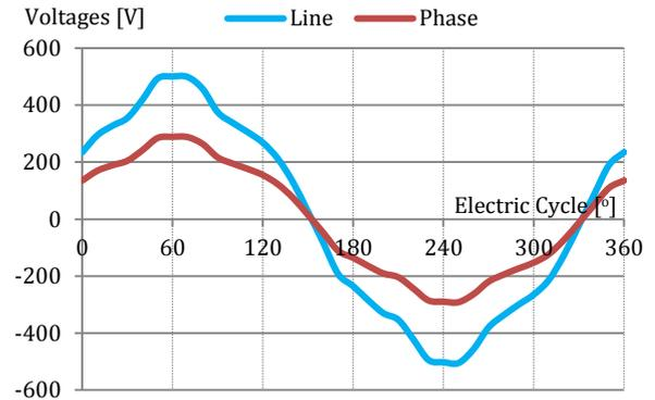
**Figure 8:** Induced voltages at 1000r/min
