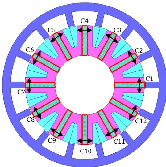
**Figure 3:** 12S-14P outer rotor PMFSM
