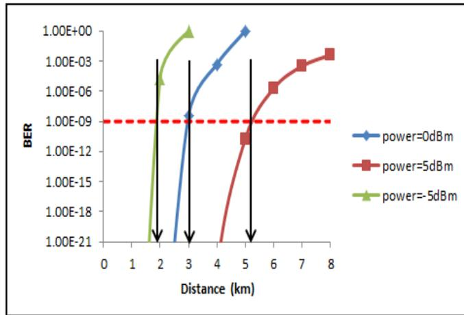
**Figure 3:** Distance versus BER performance for various power transmit level of DDM
