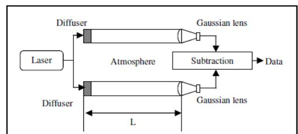
**Figure 1:** Dual Diffuser Modulation setup in FSO communication
