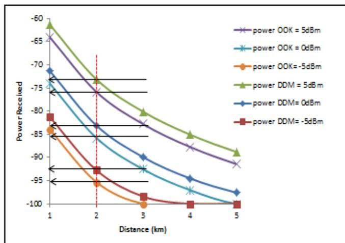
**Figure 4:** Distance versus Power Received for various power transmit level of OOK and DDM technique
