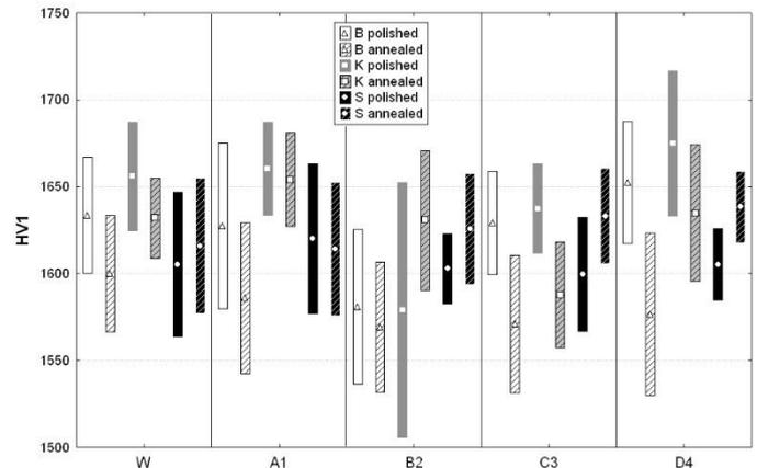
**Figure 4.** Hardness results: mean values and ±SD boxes. Solid plots are obtained after polishing, dashed ones after annealing.
