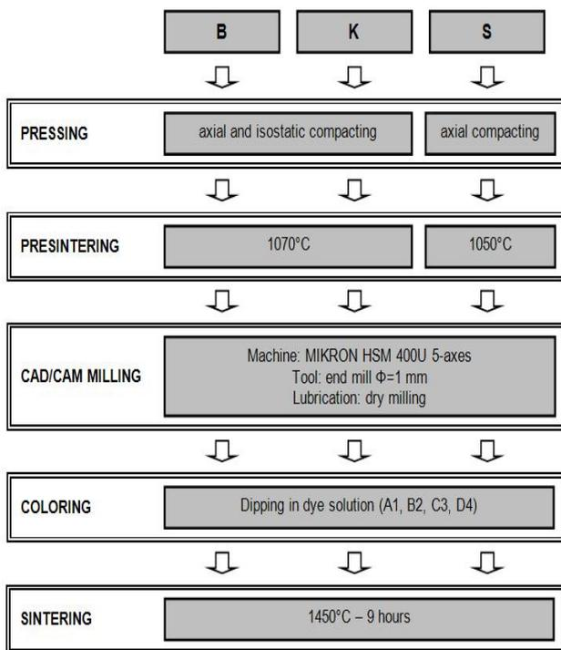
**Figure 1.** Specimens' production process
