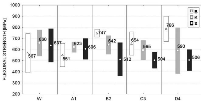
**Figure 2.** Flexural strength results: mean values and ±SD boxes.
