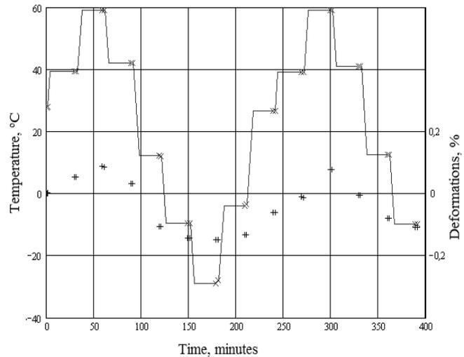
**Figure 5.** Dependency of temperature on time during the tests (red lines and symbols) and on deformation based on sample No.2 sensor 5 readings (blue symbols)
