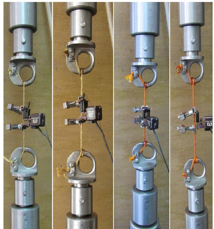
**Figure 6.** The samples of ropes made of polymer materials prior to testing at room temperature
