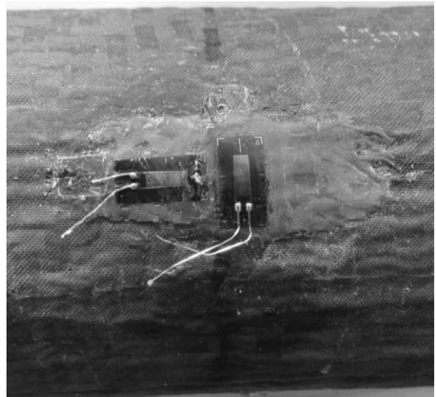
**Figure 2.** One of the areas of TKF01-5-200 type sensors attachment
