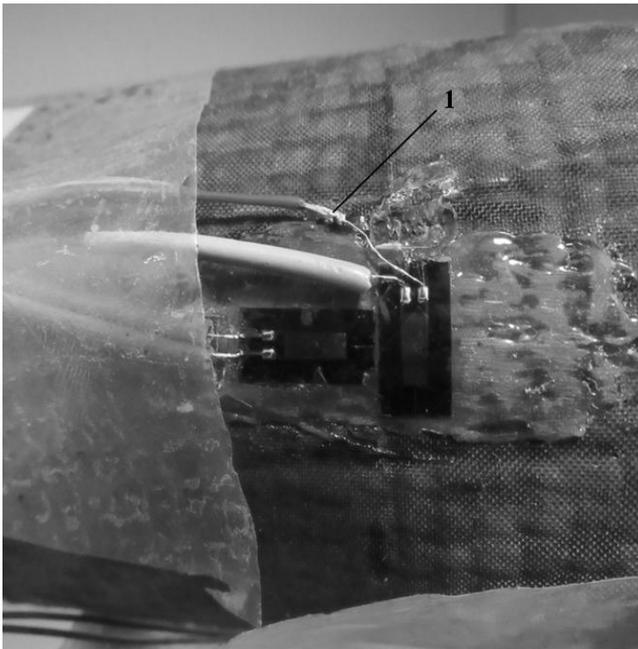
**Figure 4.** The peculiarities of connecting the sensors with the wires of the registering device (1 – seam area, insulation sleeve is moved)
