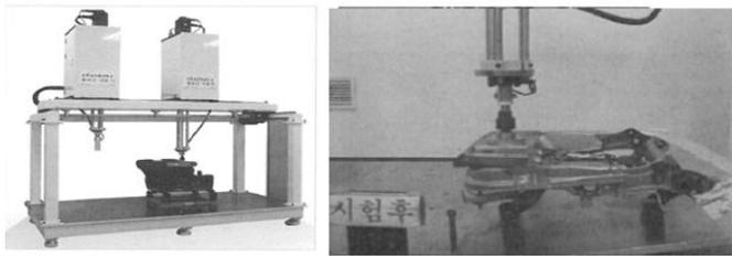
**Figure 10.** Static load tester
