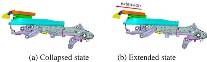
Figure 1. The Operating state of the seat extension
